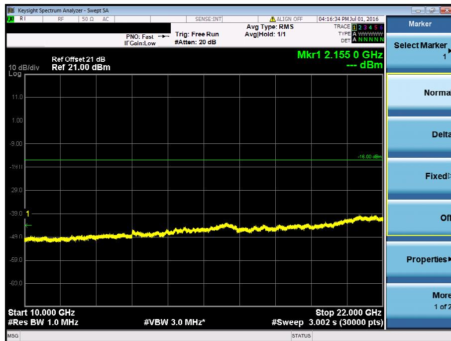
**Conducted Spurious Emission Plot on 10 MHz / M / Chain 1 / 9kHz ~ 3GHz**
