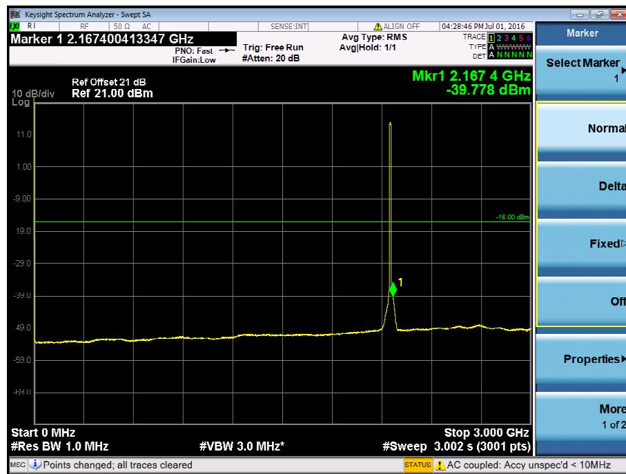
**Conducted Spurious Emission Plot on 10 MHz / T / Chain 0 / 3GHz ~ 10GHz**
