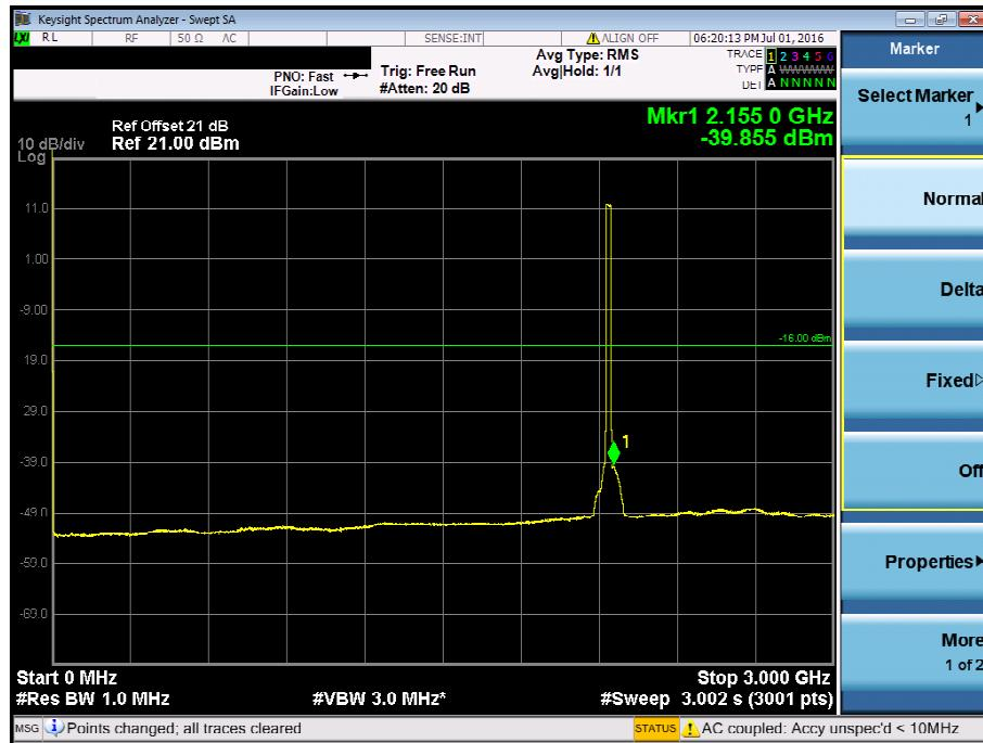
**Conducted Spurious Emission Plot on 20 MHz / M / Chain 1 / 3GHz ~ 10GHz**
