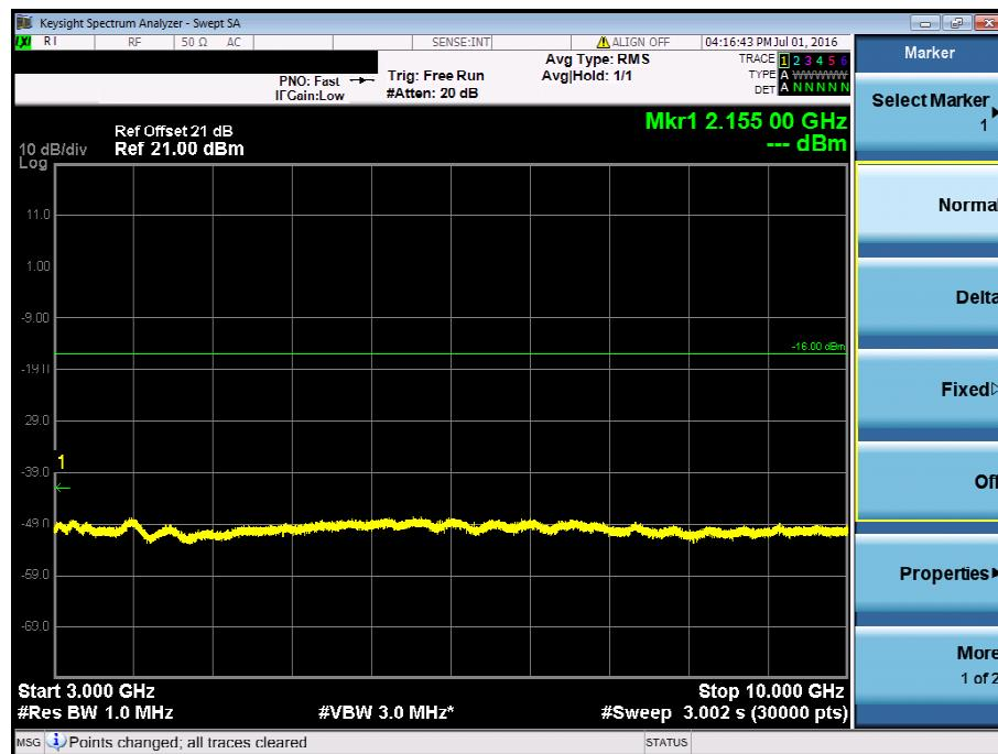
**Conducted Spurious Emission Plot on 10 MHz / M / Chain 1 / 10GHz ~ 22GHz**
