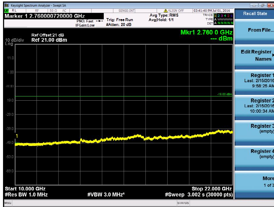
**Conducted Spurious Emission Plot on 5 MHz / T / Chain 0 / 9kHz ~ 3GHz**
