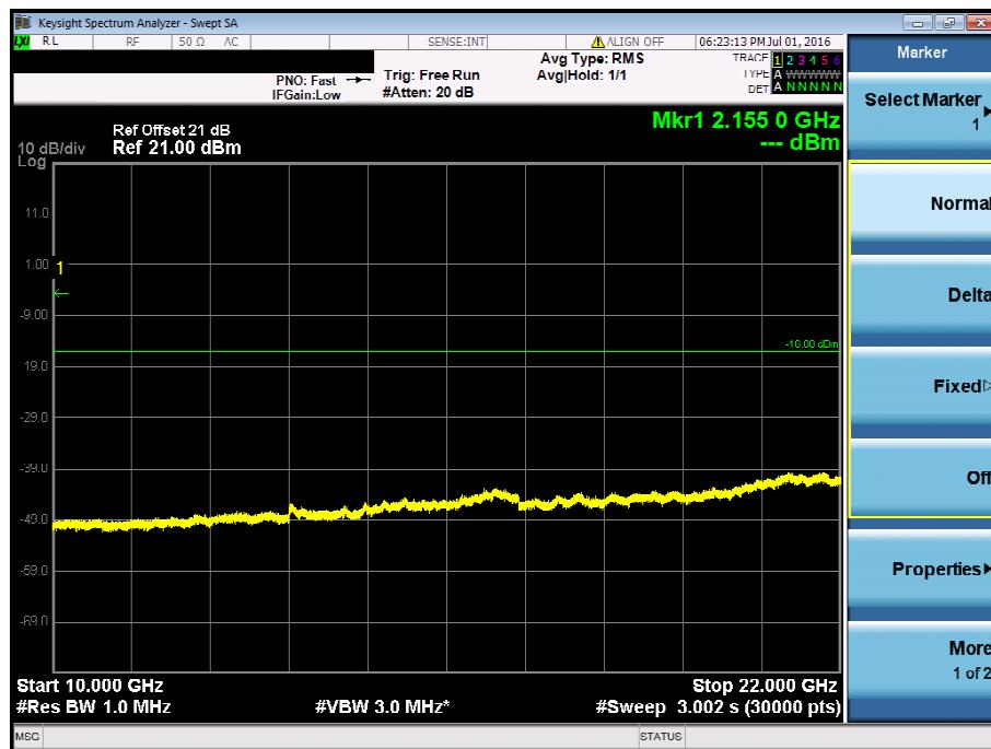
**Conducted Spurious Emission Plot on 20 MHz / T / Chain 1 / 9kHz ~ 3GHz**
