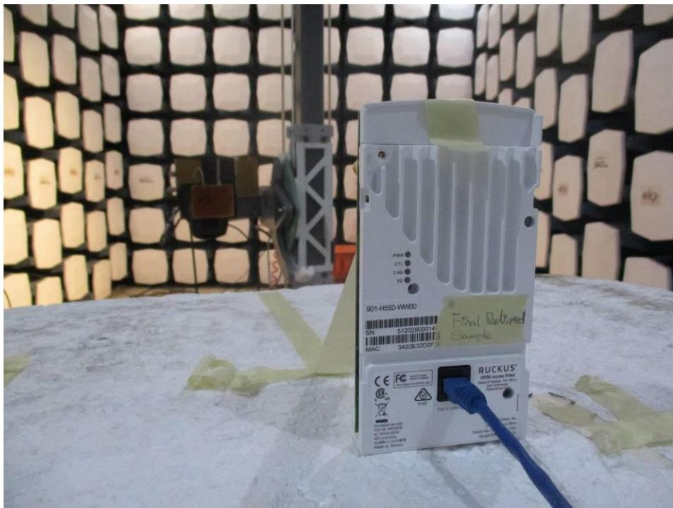
**1.9 18 – 26.5-40 GHz at 1 Meter Front View**
