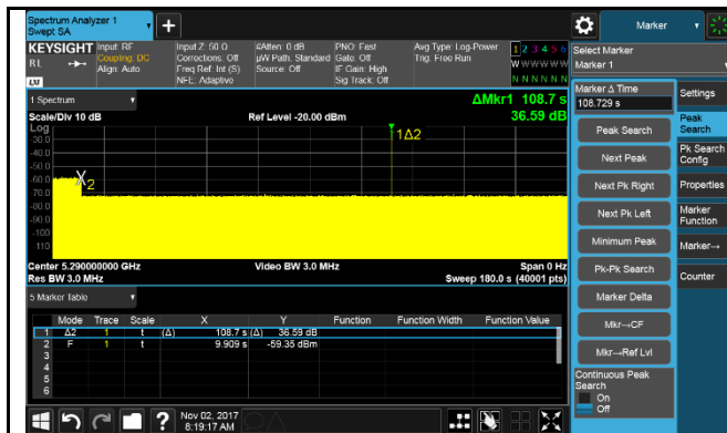
Radar at end of CAC – VHT80 – 5290MHz
