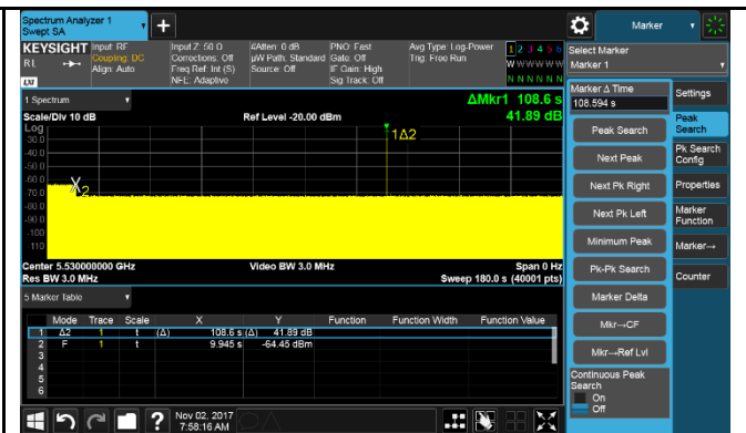
Radar at end of CAC – VHT80 – 5530MHz
