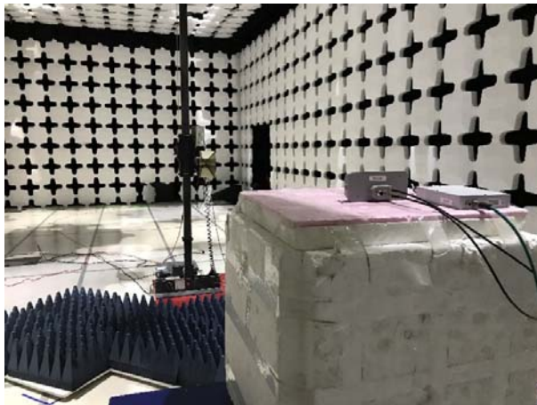
Radiated Emissions (>1GHz) – Front View
