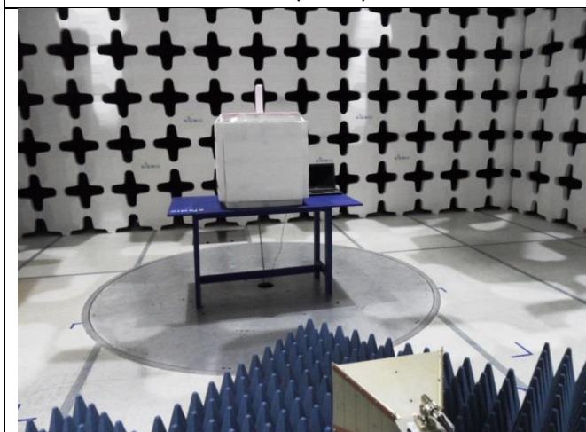
Radiated Emissions (>1GHz) – Front View
