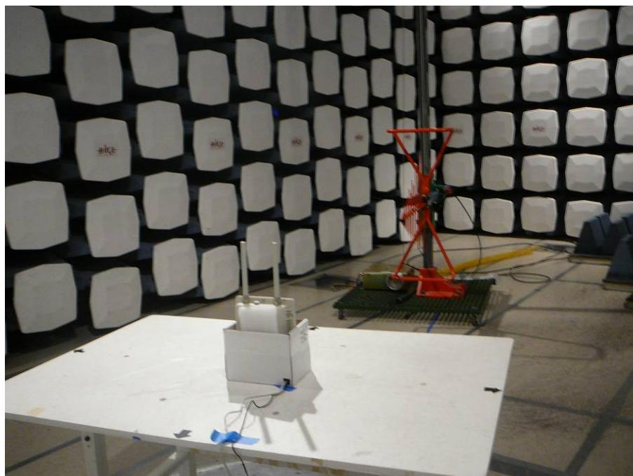
**15.3 Radiated Emission above 1 GHz Front View**
