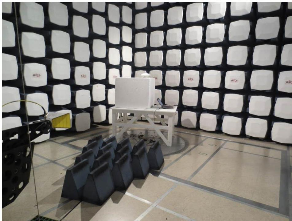
**14.12 Radiated Emission 3 dBi Antenna above 1 GHz Rear View**
