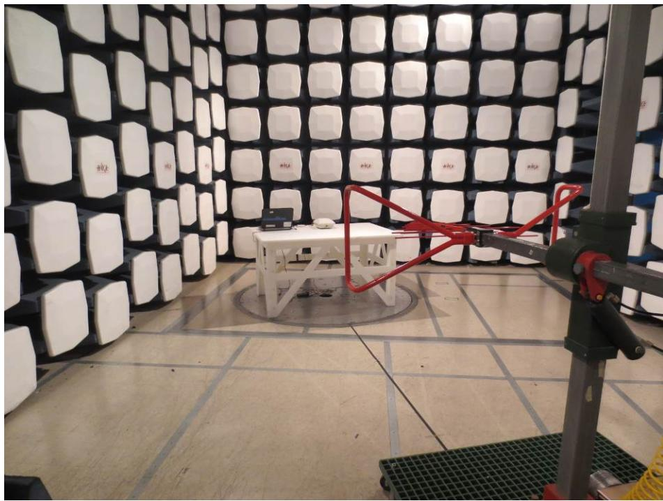
**14.10 Radiated Emission 15 dBi Antenna below 1 GHz Rear View**
