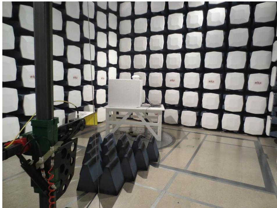
**14.20 Radiated Emission 15 dBi Antenna above 1 GHz Rear View**
