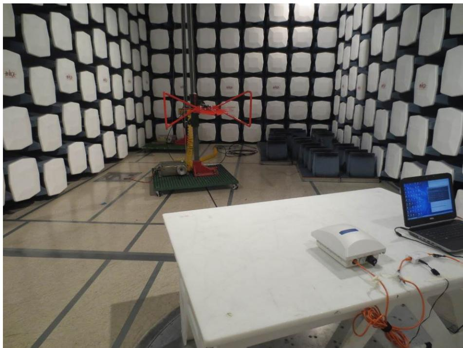
**14.11 Radiated Emission 3 dBi Antenna above 1 GHz Front View**
