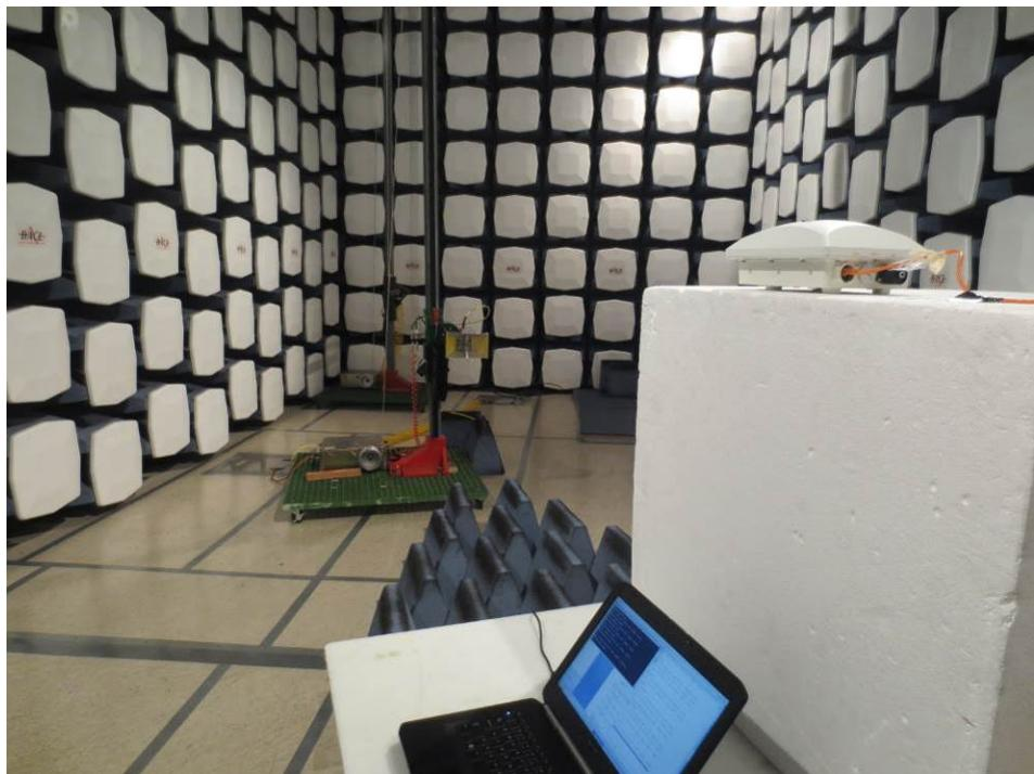
**14.17 Radiated Emission 12 dBi Antenna above 1 GHz Front View**
