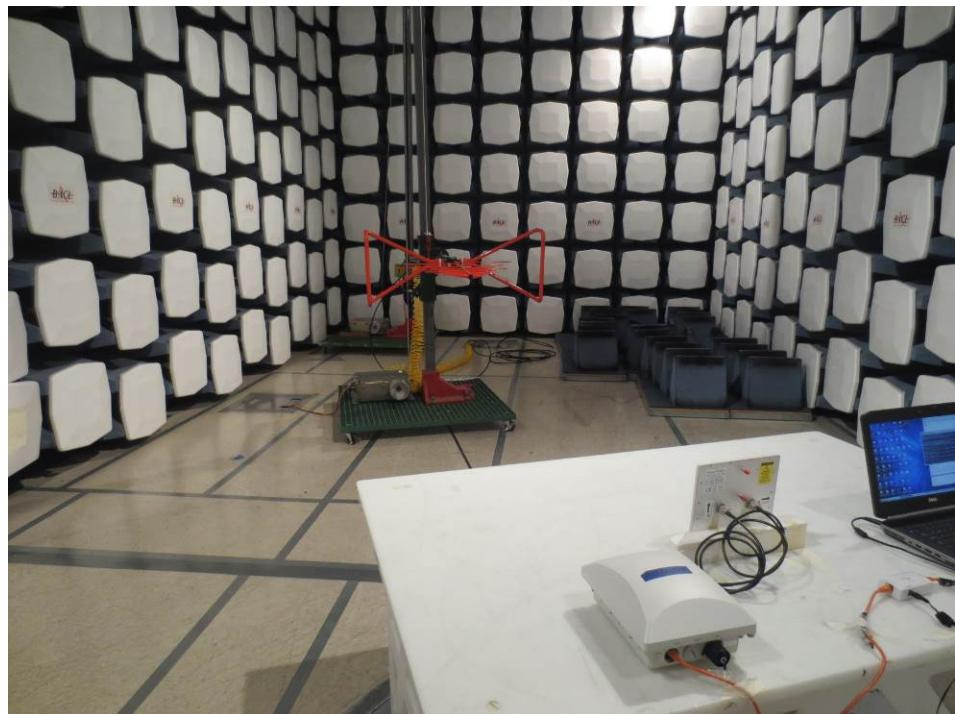
**14.9 Radiated Emission 15 dBi Antenna below 1 GHz Front View**
