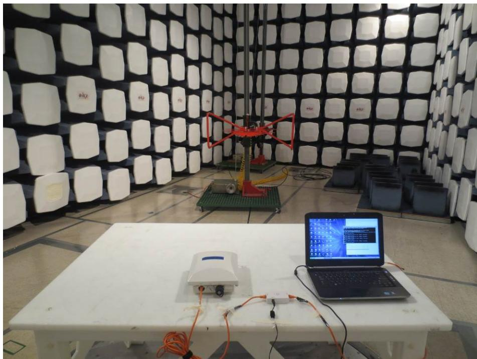
**14.7 Radiated Emission 12 dBi Antenna below 1 GHz Front View**
