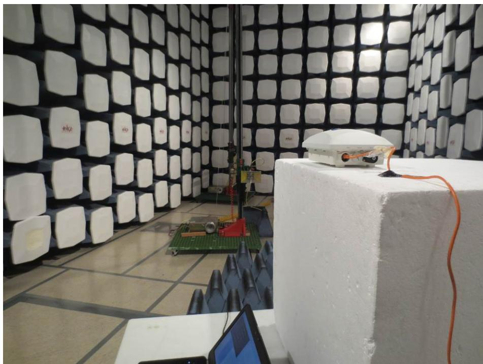
**14.13 Radiated Emission 5 dBi Antenna above 1 GHz Front View**
