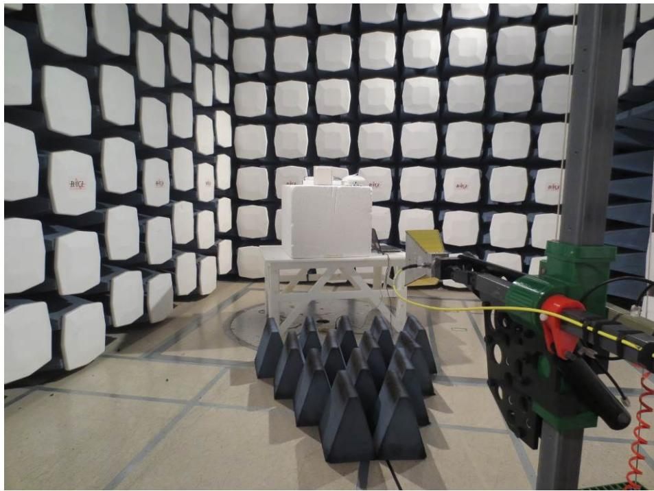
**14.18 Radiated Emission 12 dBi Antenna above 1 GHz Rear View**
