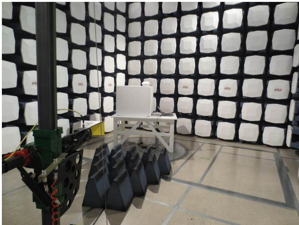
**14.16 Radiated Emission 8 dBi Antenna above 1 GHz Rear View**
