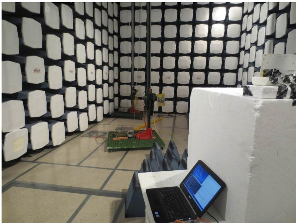
**14.15 Radiated Emission 8 dBi Antenna above 1 GHz Front View**
