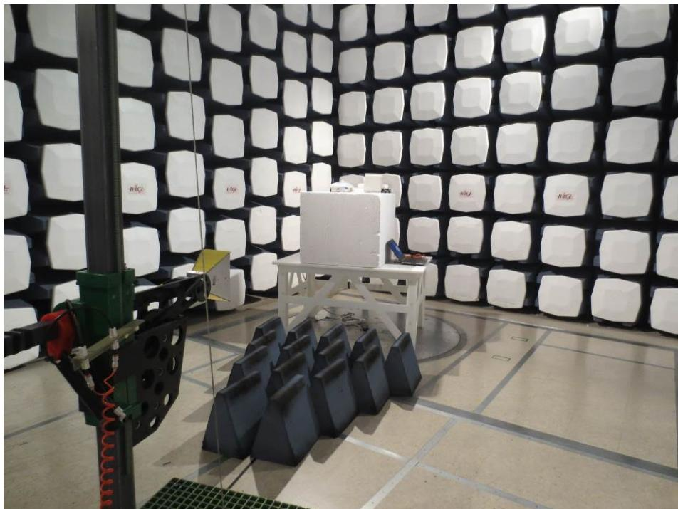
**14.14 Radiated Emission 5 dBi Antenna above 1 GHz Rear View**
