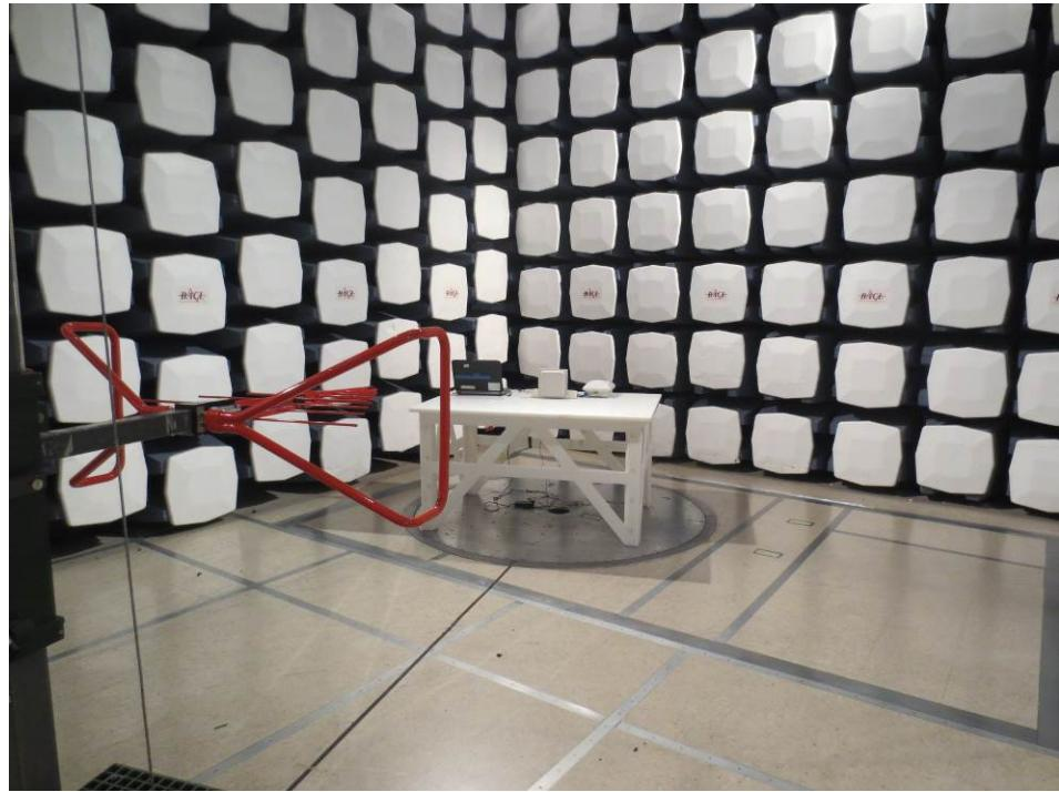
**14.8 Radiated Emission 12 dBi Antenna below 1 GHz Rear View**
