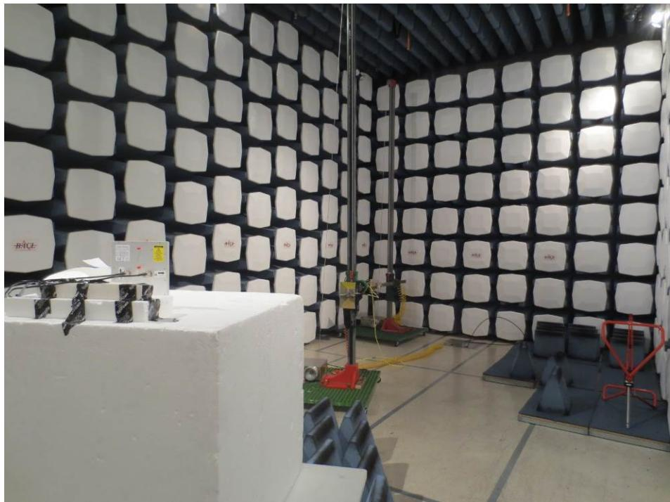
**14.19 Radiated Emission 15 dBi Antenna above 1 GHz Front View**
