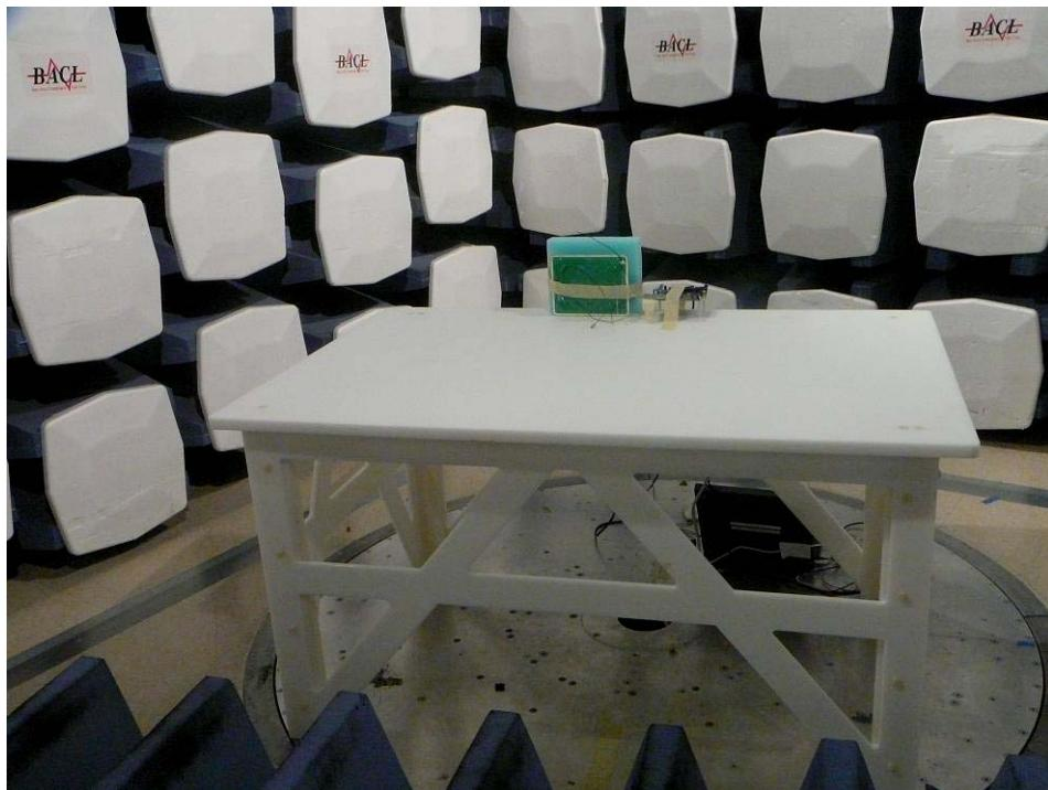
**12.5 Radiated Emission below 1 GHz Rear View @ 15 dBi Antenna - TBolt2**
