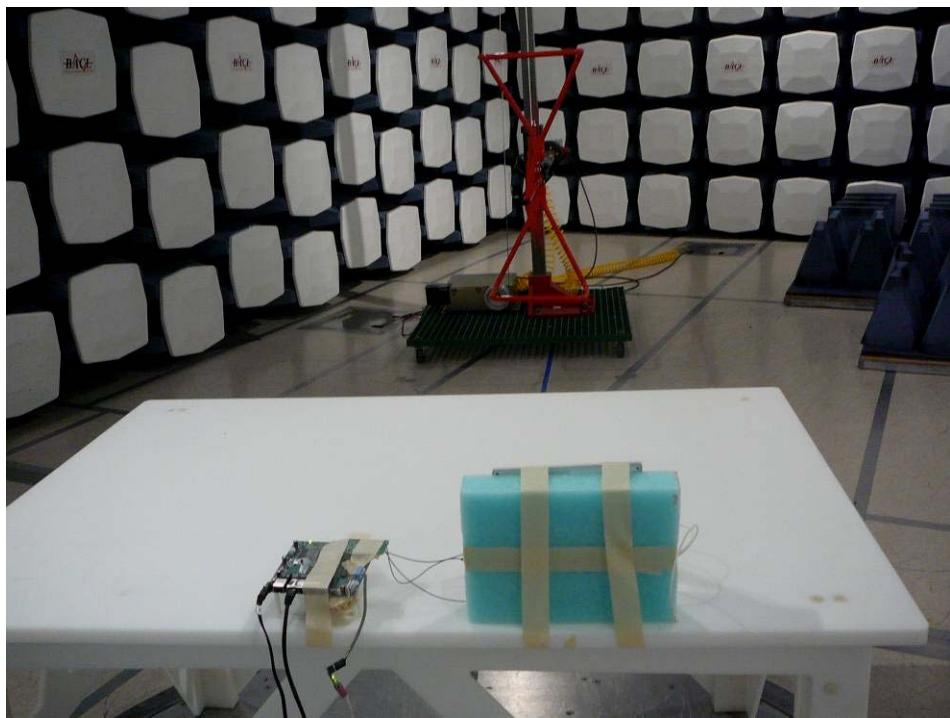
**12.3 Radiated Emission above 1 GHz Rear View @ 5 dBi Antenna - AT-0505-MP**
