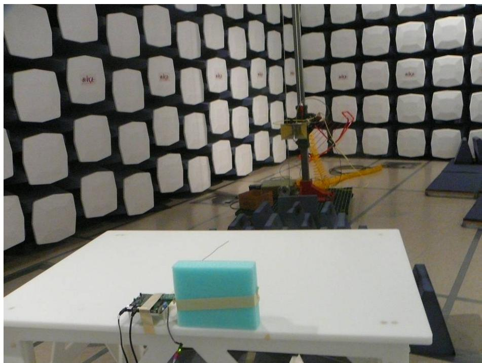
**12.7 Radiated Emission Front View @ 5 dBi Antenna – AT-0636-VP**
