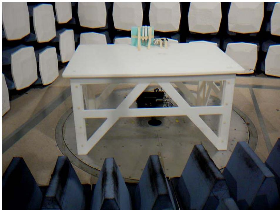
**12.8 Radiated Emission below 1 GHz Rear View @ 5 dBi Antenna – AT-0636-VP**
