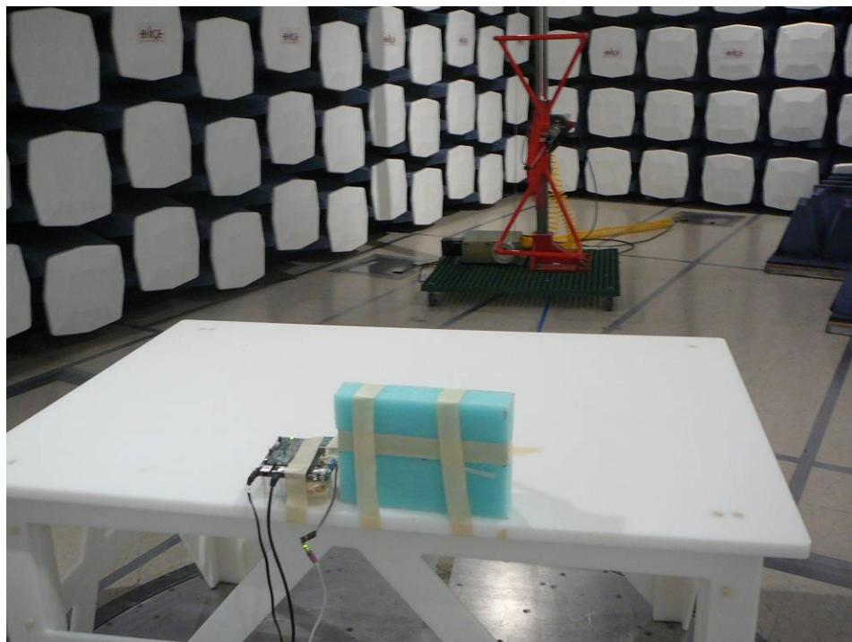
**12.6 Radiated Emission above 1 GHz Rear View @ 15 dBi Antenna - TBolt2**
