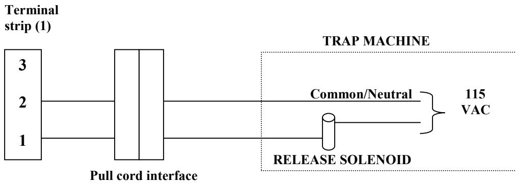
**NOTE:** NEVER wire to pin 3 of the terminal strip without FIRST contacting E R A D. (817-244-1761 or [erad@flash.net](mailto:erad@flash.net))
