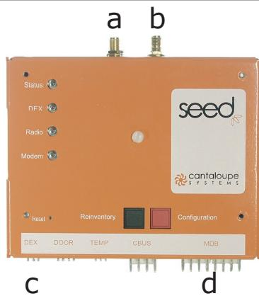
Plug in the cables to the seed device. Refer to the diagram on the left for reference.
