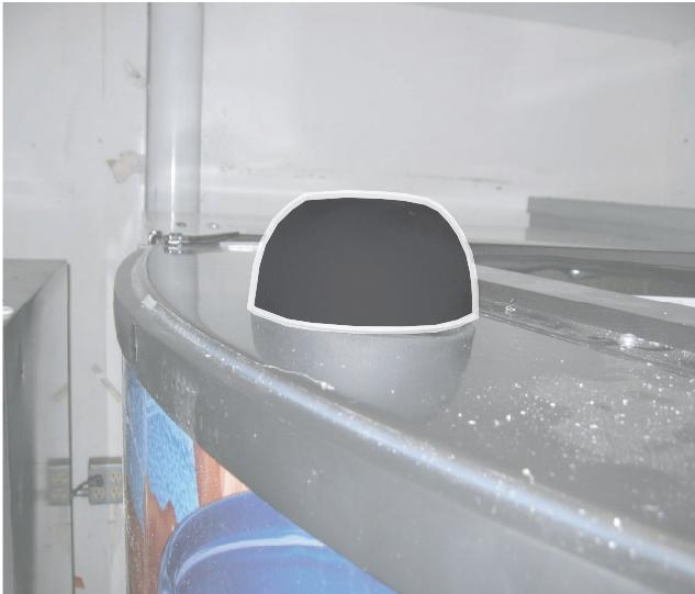
1. Position the antenna on top of the machine. We recommend mounting it on the part of the machine where the vending machine controller is attached to. We recommend putting it as center and far forward as possible. The example to the left is mounted on the door.
