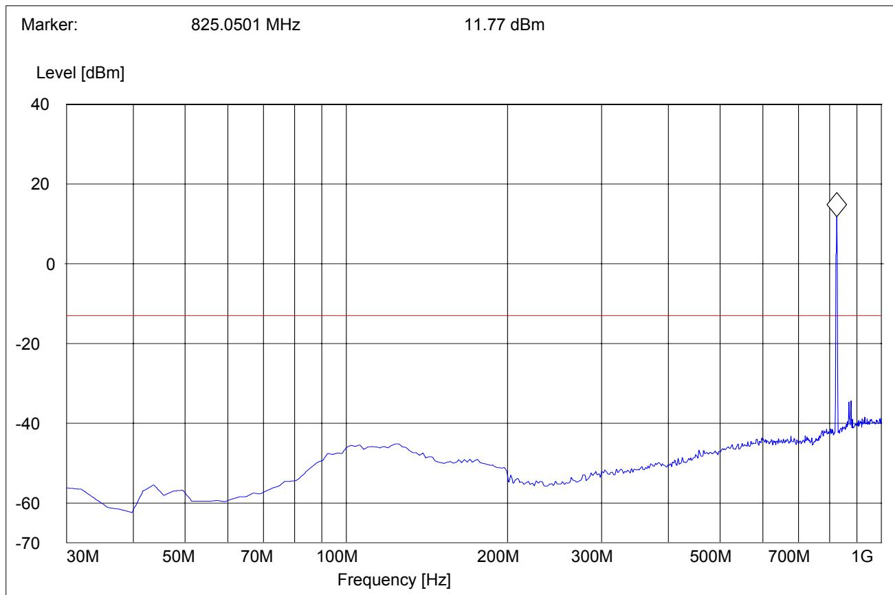
**RADIATED SPURIOUS EMISSIONS (GSM-850)****30MHz - 1GHz**
