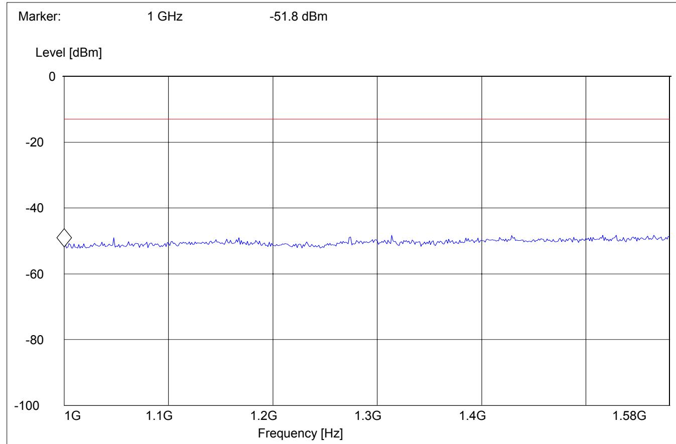
**RADIATED SPURIOUS EMISSIONS (GSM-850)****Tx @ 848.8MHz: 1.58GHz – 3GHz**
