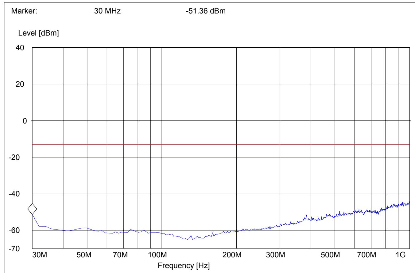
**RADIATED SPURIOUS EMISSIONS (IDLE MODE)****EUT in Idle Mode: 1GHz – 3GHz**
