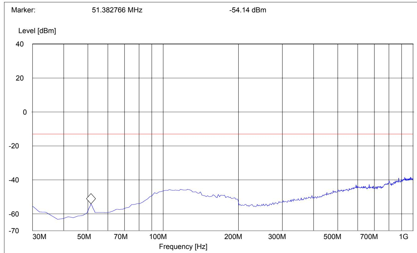
**RADIATED SPURIOUS EMISSIONS (IDLE MODE)****EUT in Idle Mode: 30MHz – 1GHz**
