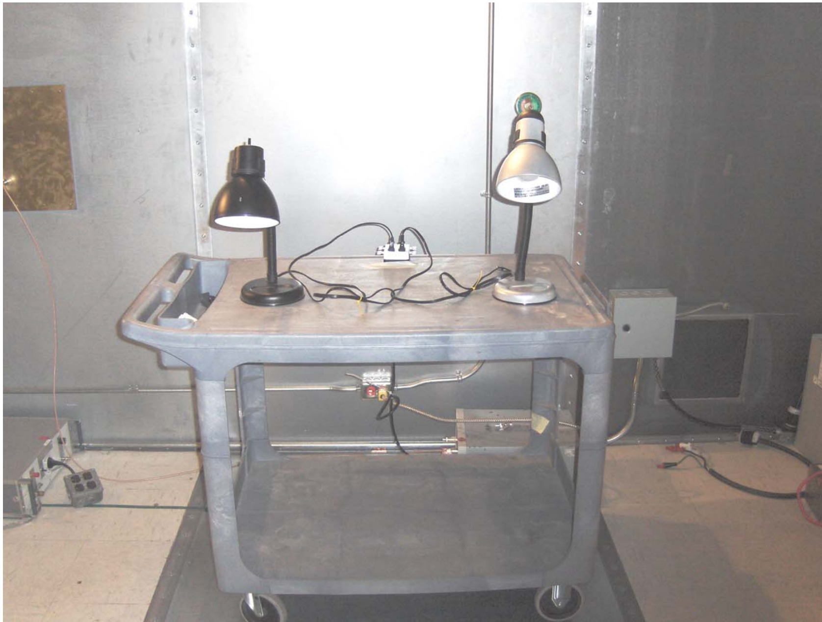
Photo #1: AC Conducted Emissions Measurements
