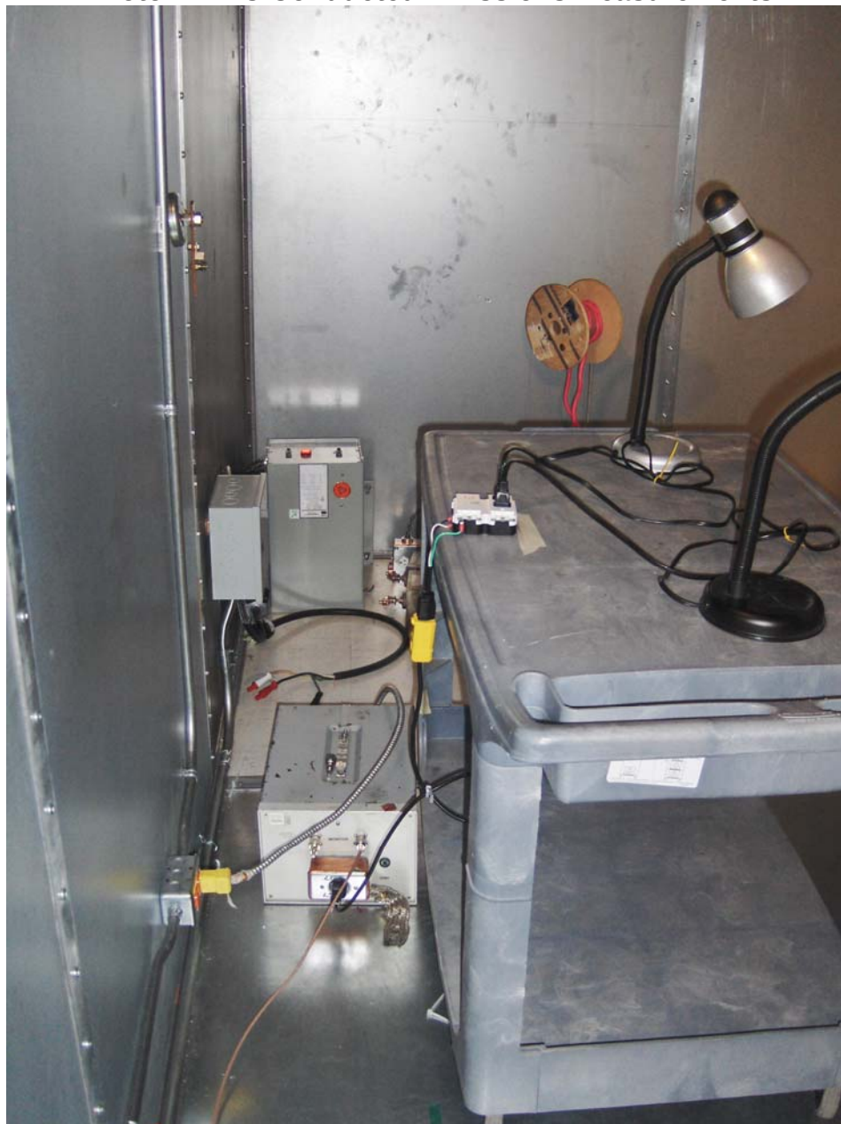
Photo #2: AC Conducted Emissions Measurements
