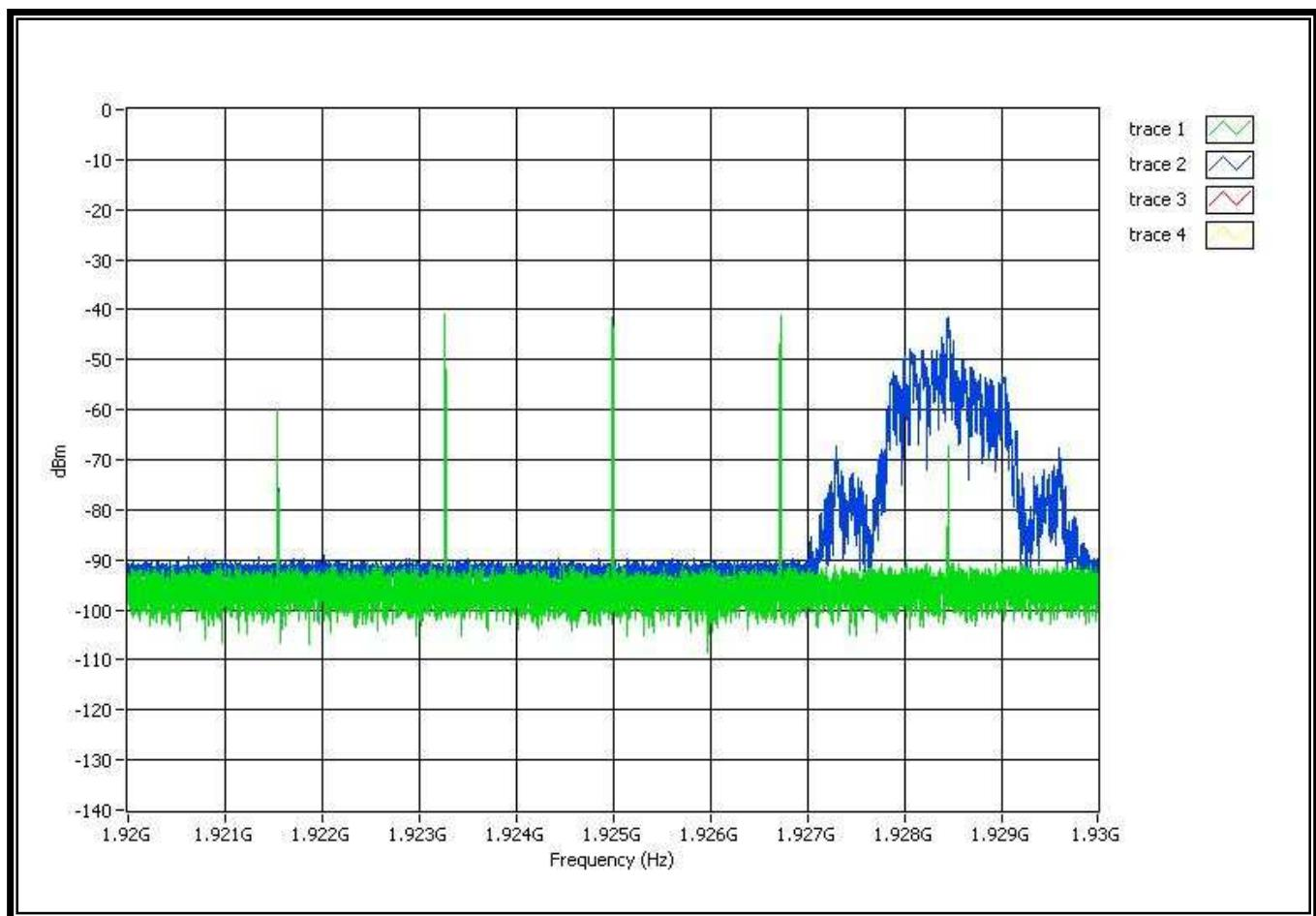
Note 1: The interference of level on f1 is TL+UM+1dB. The interference of level on f2 is TL+UM-6dB. The level of other 3 carriers is TU+UM.
