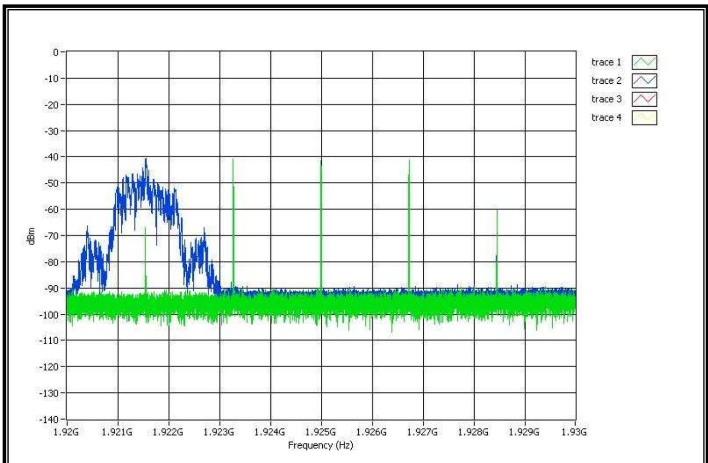
Note 1: The interference of level on f2 is TL+UM+1dB. The interference of level on f1 is TL+UM-6dB. The level of other 3 carriers is TU+UM.
