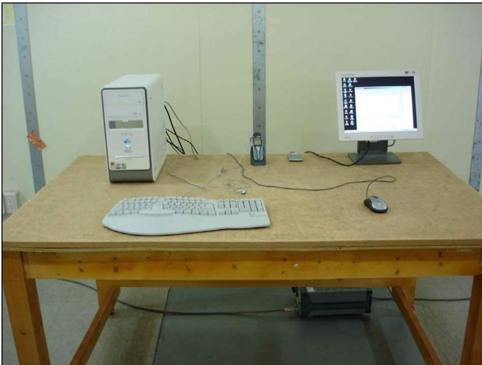
Photograph 1: Setup for Conducted Emissions [PC Download Mode]
