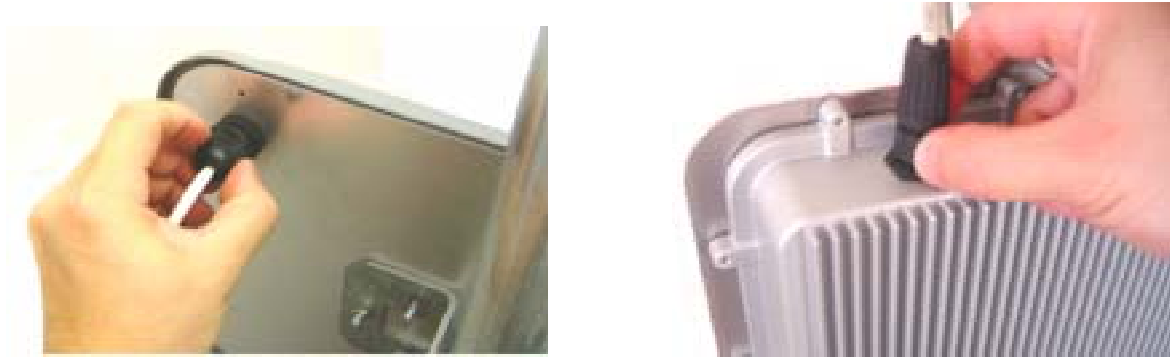
Figure 14. Tighten the Cable through Water Prof Connector: : Integrated ODU (Left) and Non-Integrated ODU (Right)
