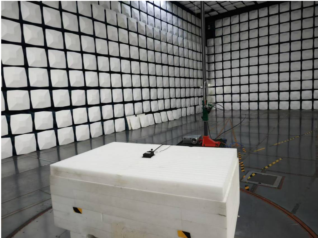
Radiated Emission 9k-30MHz Perpendicular View
