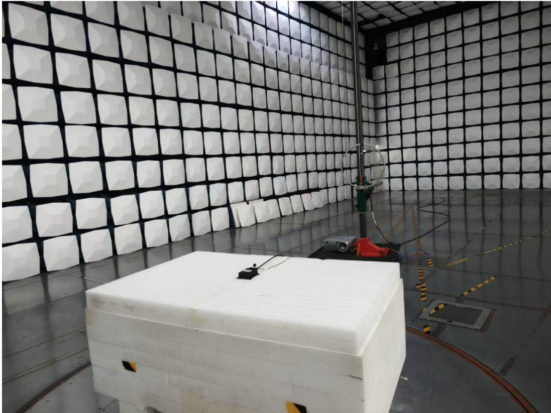
Radiated Emission 9k-30MHz Perpendicular View
