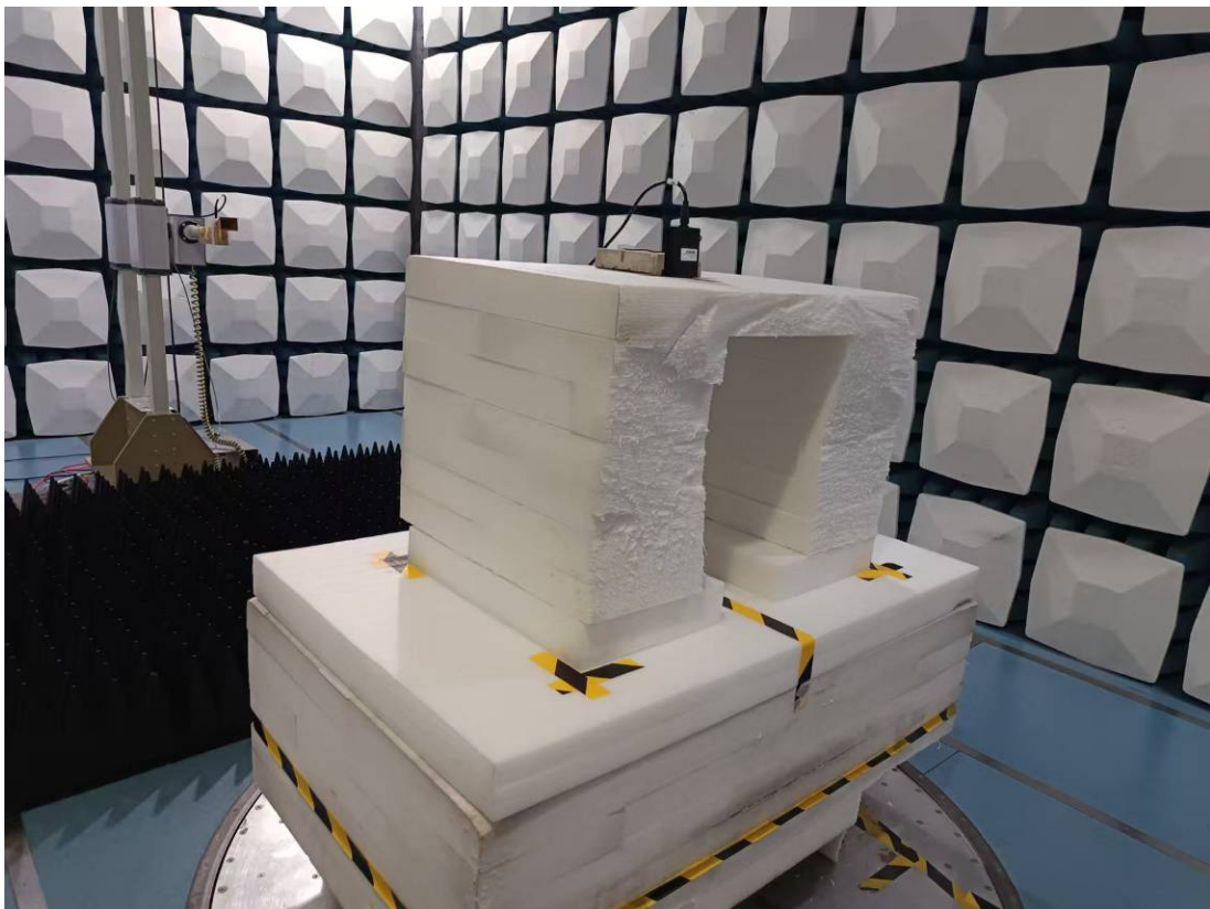
Radiated Emission 18-25GHz View
