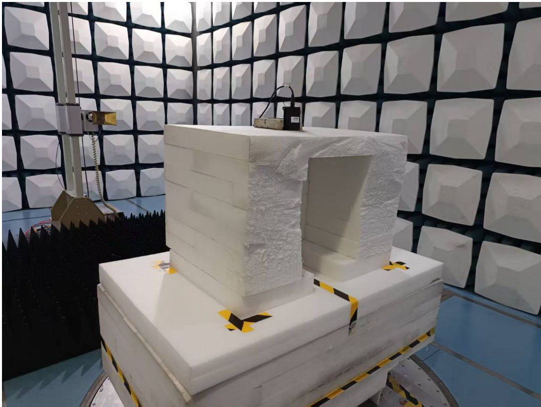
Radiated Emission 18-25GHz View
