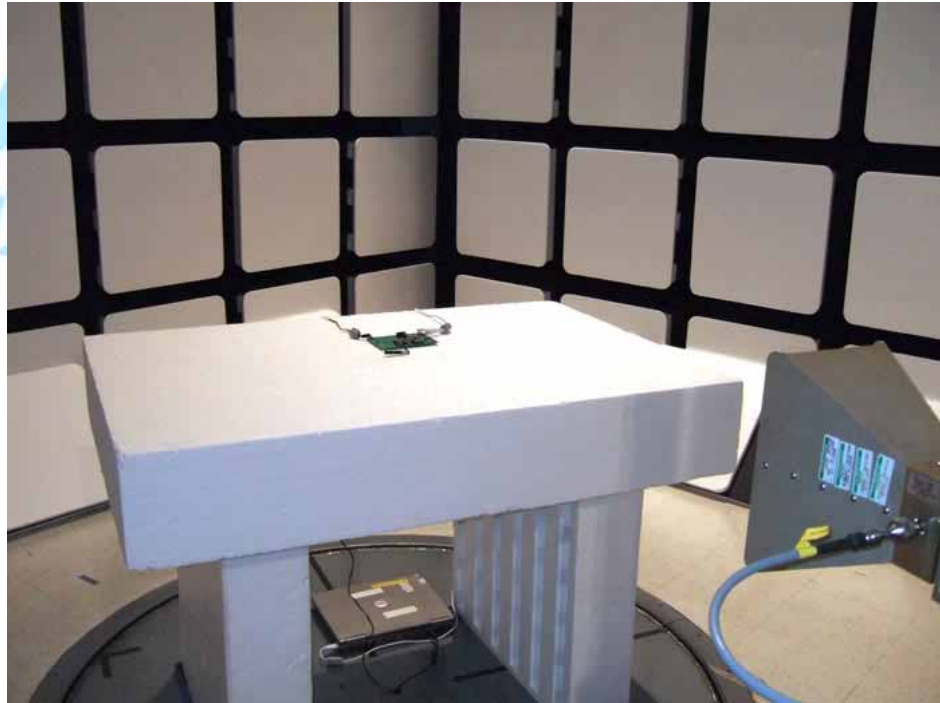
Test Configuration 2: 960 MHz – 40 GHz
