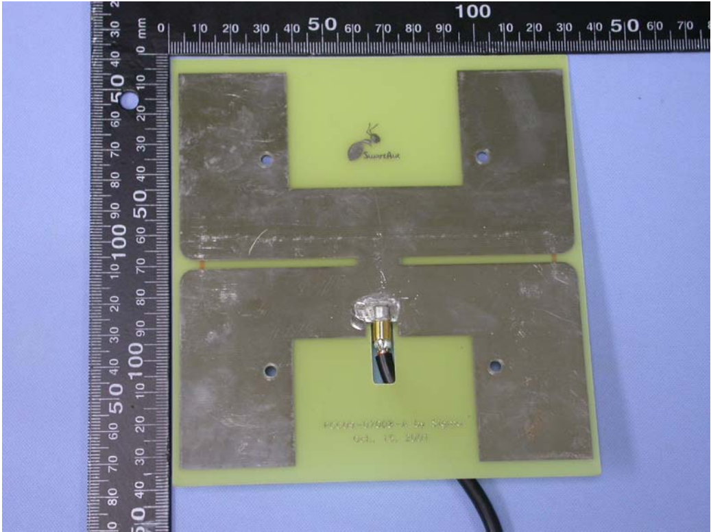
11. Front view of PCB (A9235-A-002-NET)
