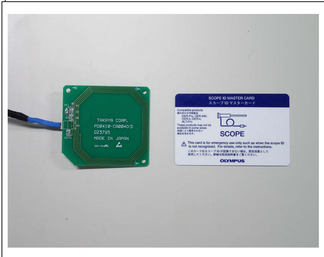
Scope ID master card & RFID Antenna
