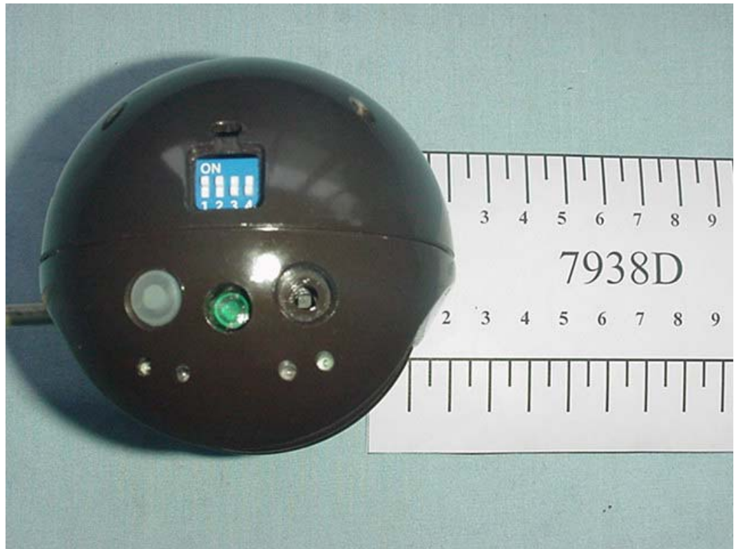
FIGURE 5 MOTION SENSOR WITH RF TRANSMITTER (M/N: 7938D) TRANSMITTER (TOP VIEW)
