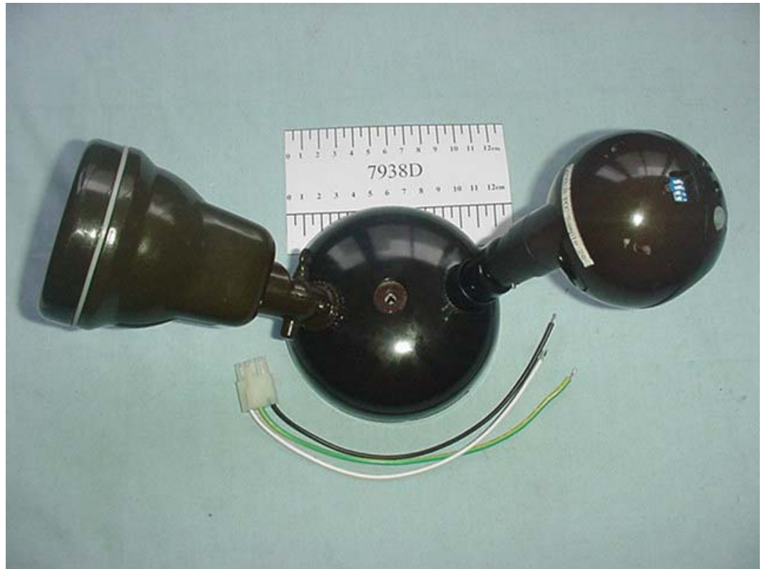
FIGURE 1 MOTION SENSOR WITH RF TRANSMITTER (M/N: 7938D) GENERAL APPEARANCE (TOP VIEW)
