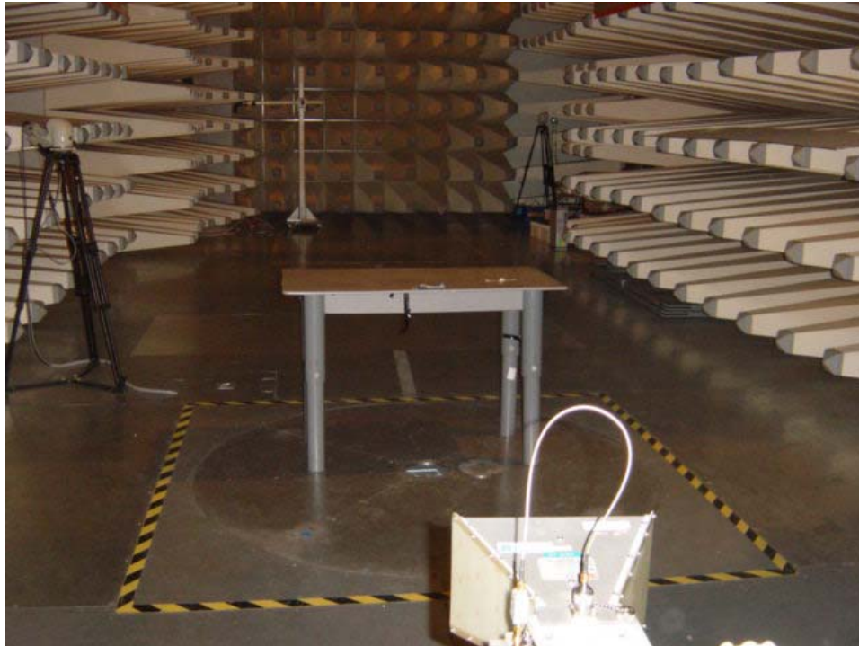
Set-up for Radiation Emission (Transmitter)
