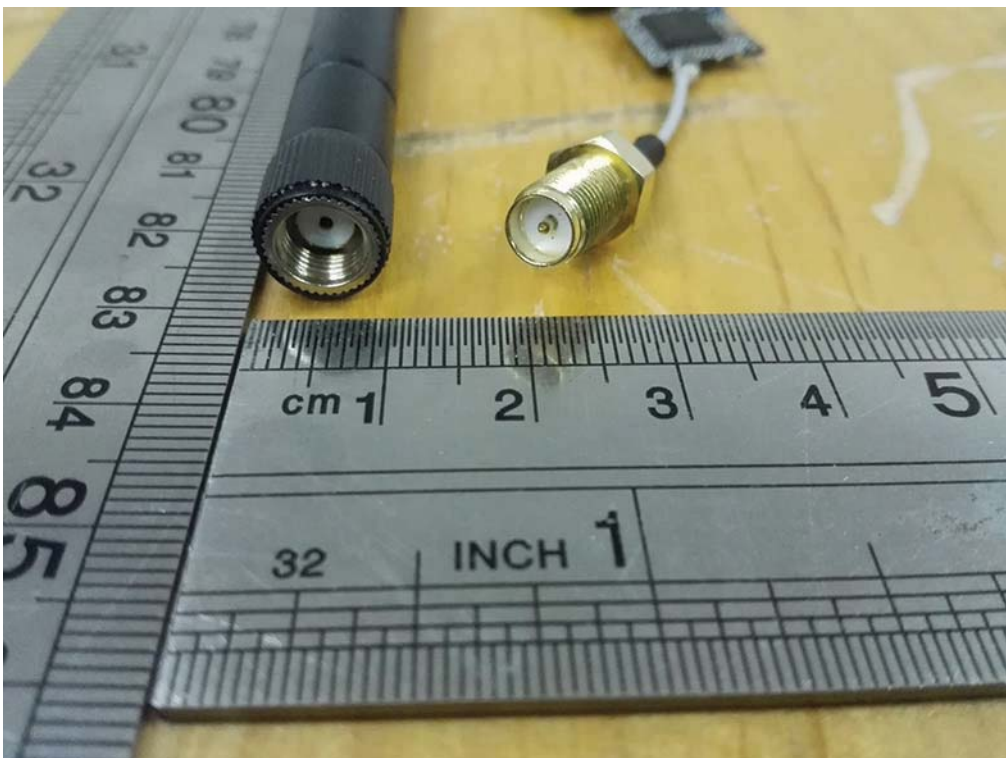
Reversed polarity non standard antenna port
