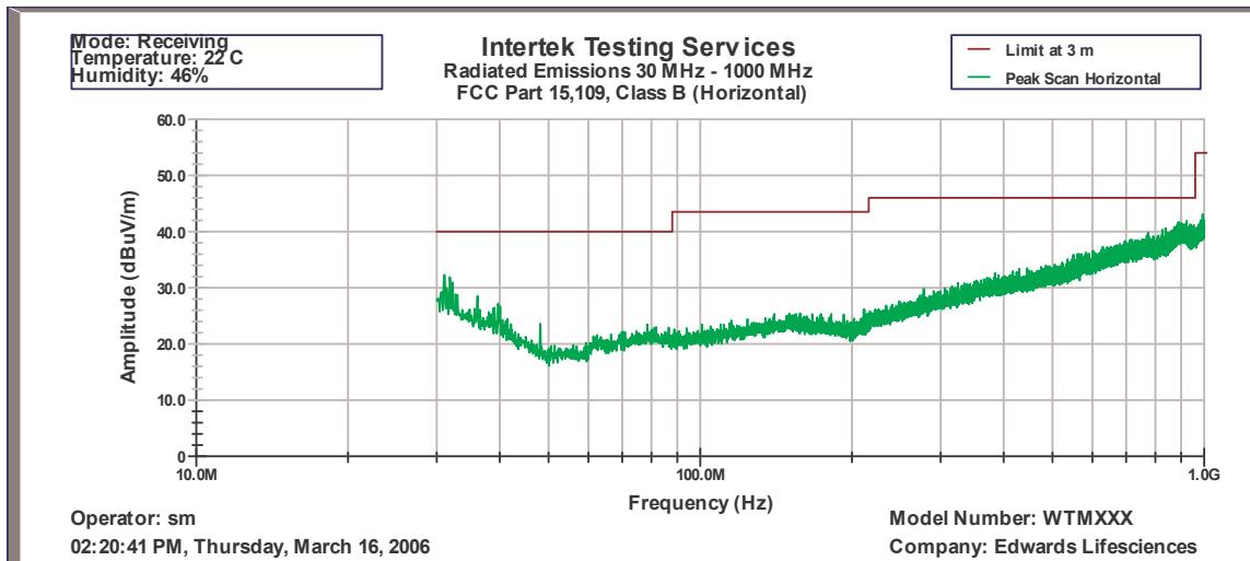
**Radiated Emission, M Unit, Horizontal Polarization**
