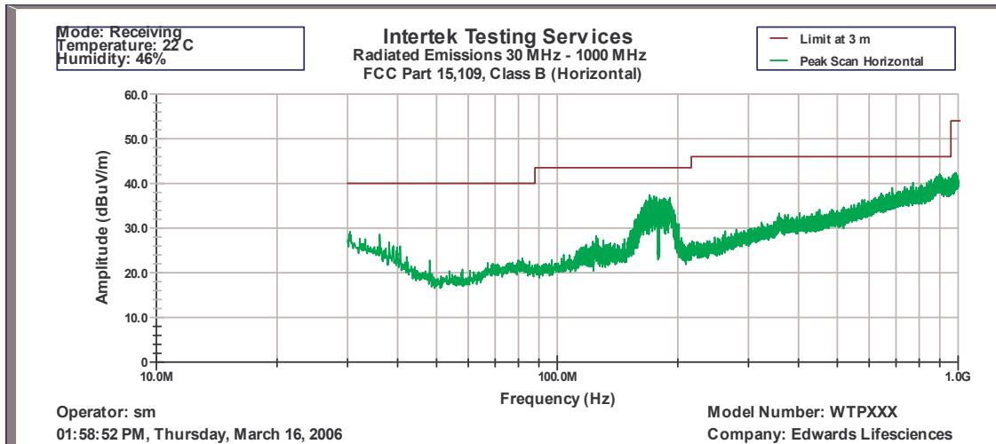
**Radiated Emission, X Unit, Horizontal Polarization**
