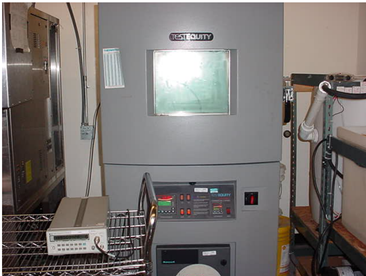
X / M Unit, Frequency Stability Test vs. Temperature
