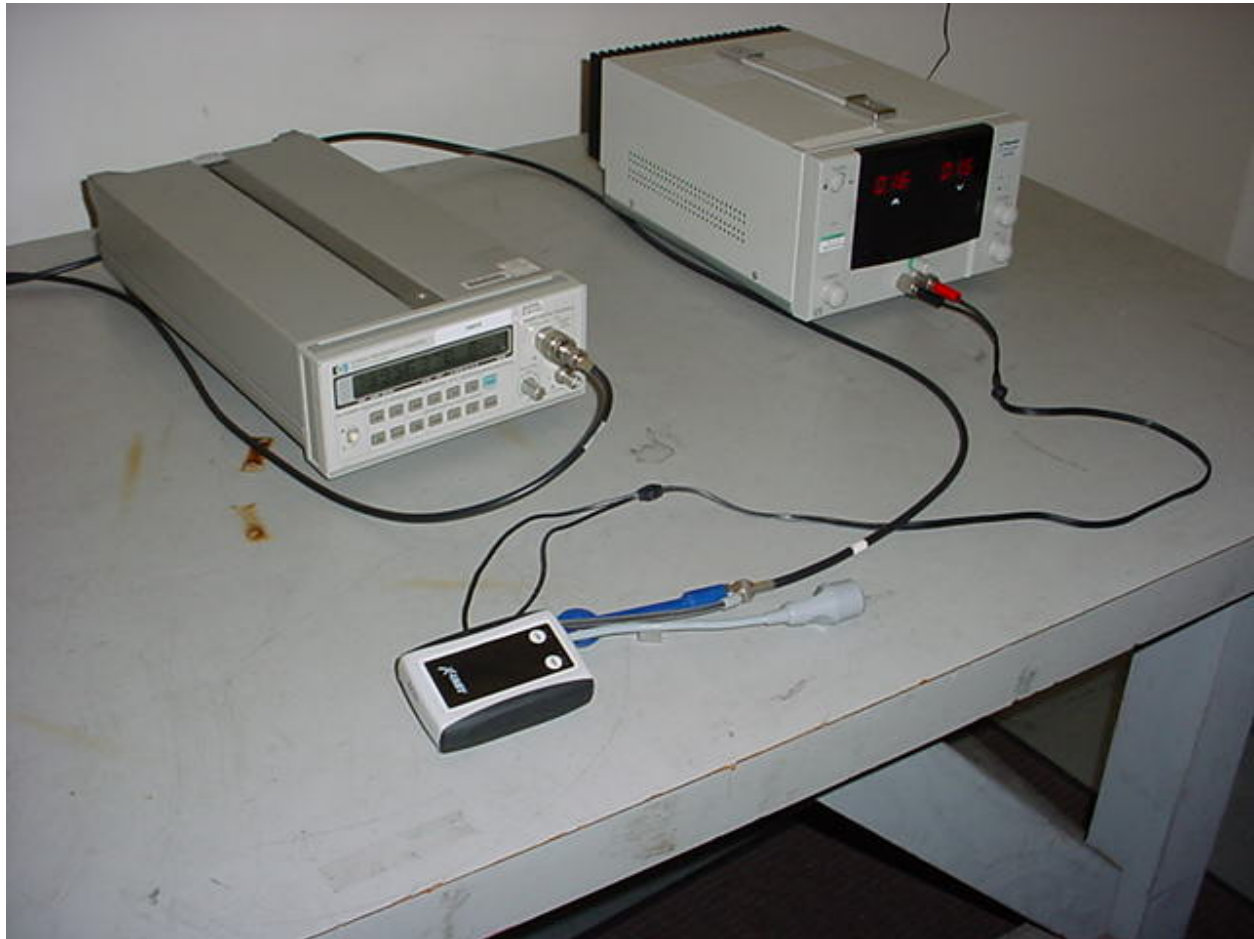
X Unit, Temperature Stability vs. Voltage
