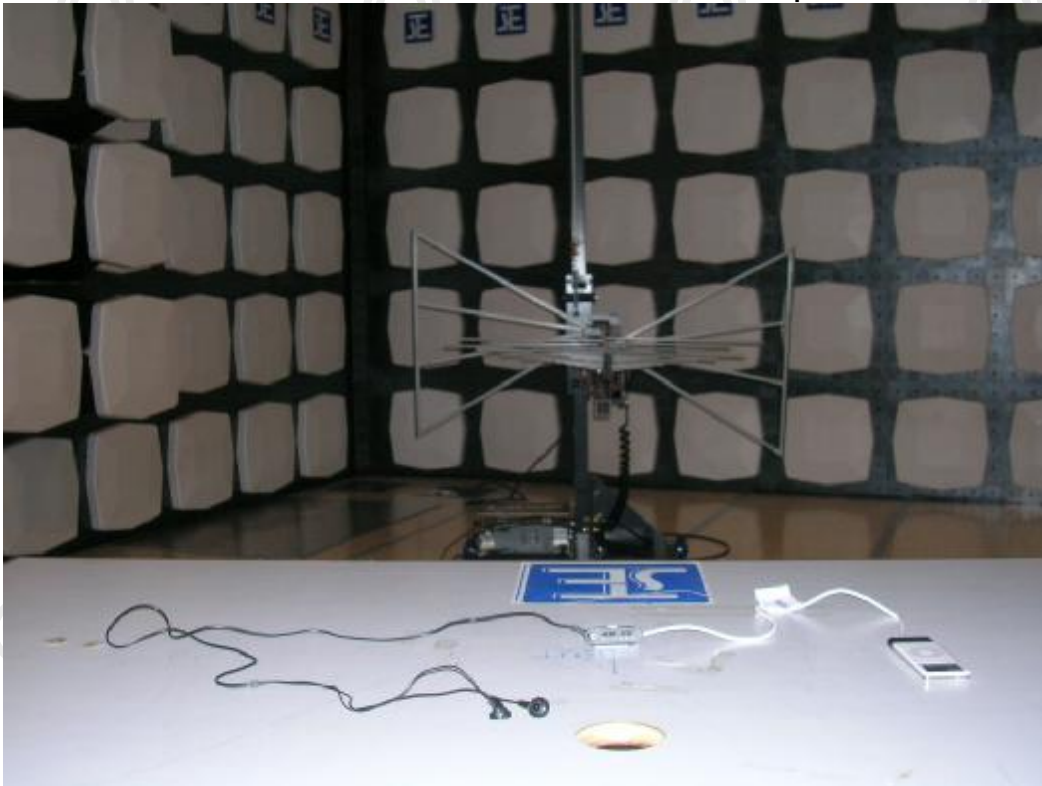
Measurement of Radiated Emission Test Set Up
