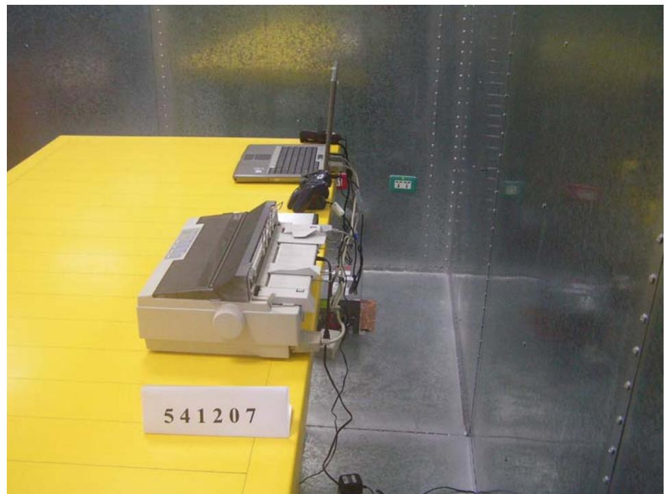
5.3.11. Photographs of Radiated Emission Test Configuration
