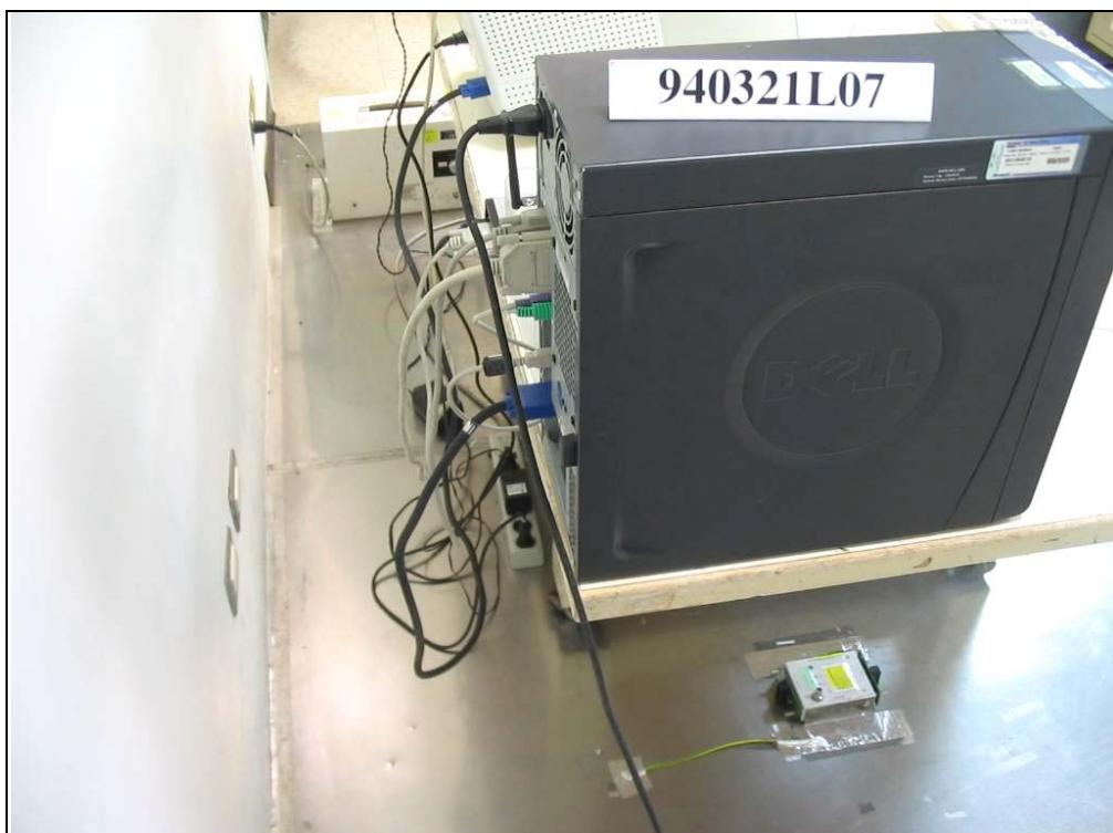
**RADIATED EMISSION TEST (Below 1 GHz, antenna with antenna cable)**
