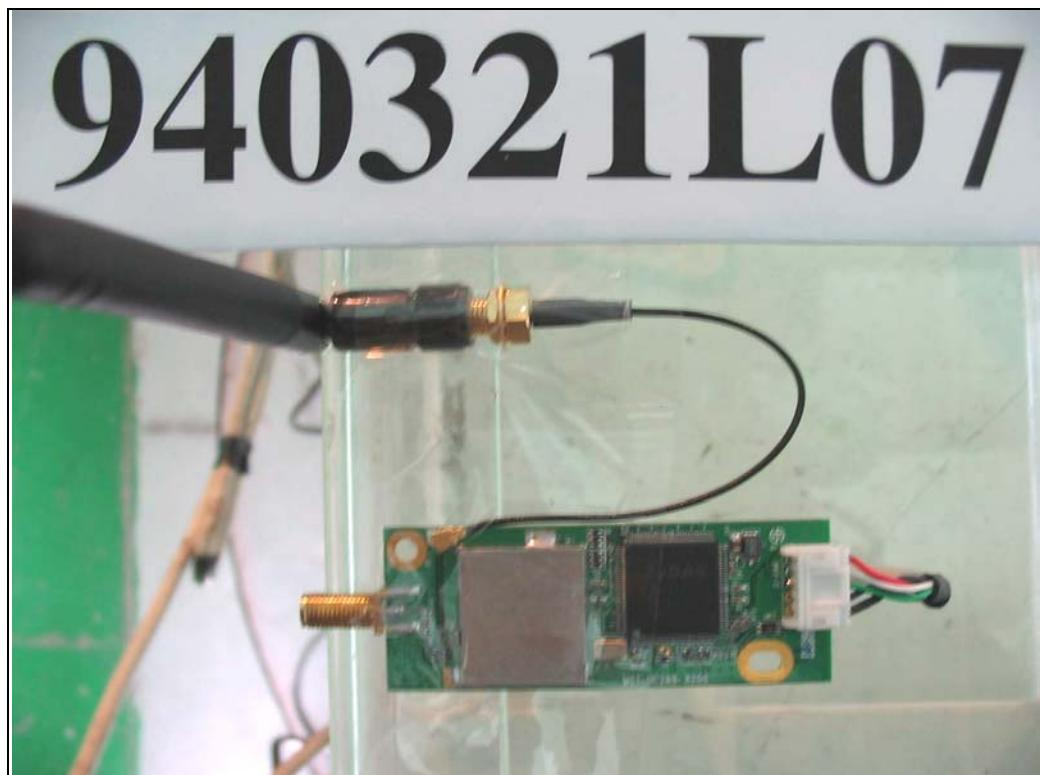
**RADIATED EMISSION TEST (Above 1 GHz, antenna without antenna cable)**
