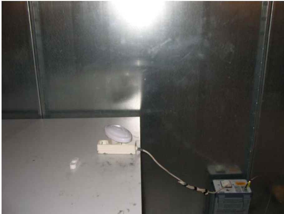
Conducted Emission Test
