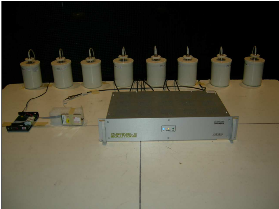
Figure 1: Radiated Emissions – Ceiling Mount Antenna
