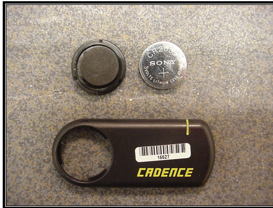
PHOTOGRAPH 14: TRANSMITTER COVER AND BATTERY
