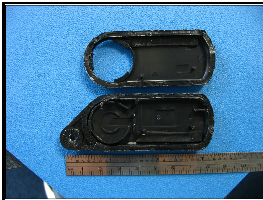
PHOTOGRAPH 13: TRANSMITTER FRONT AND BACK COVER - INSIDE VIEW
