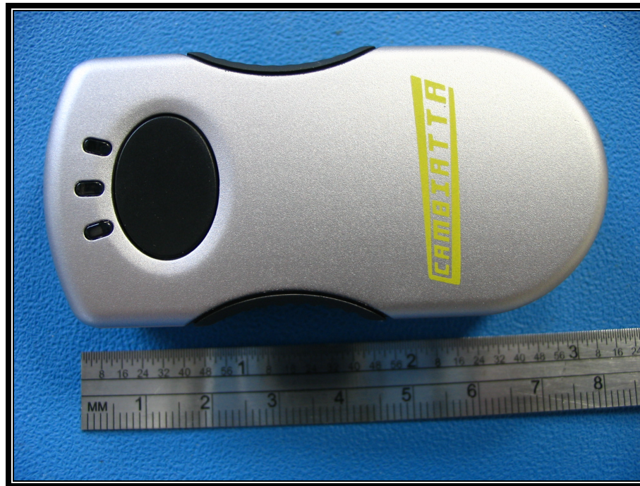
PHOTOGRAPH 6: DATA LOGGER FRONT VIEW
