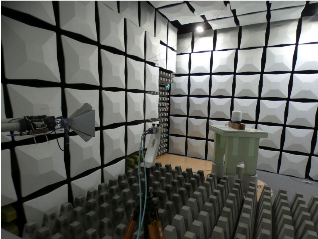
Photo 7: Test setup for radiated measurements (fully-anechoic chamber, > 40 GHz, FCC, Measurement distance: 3m)
