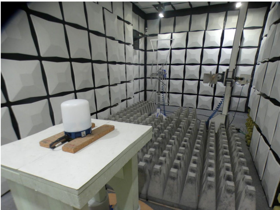
Photo 4: Test setup for radiated measurements (fully-anechoic chamber, 1 GHz – 26 GHz)
