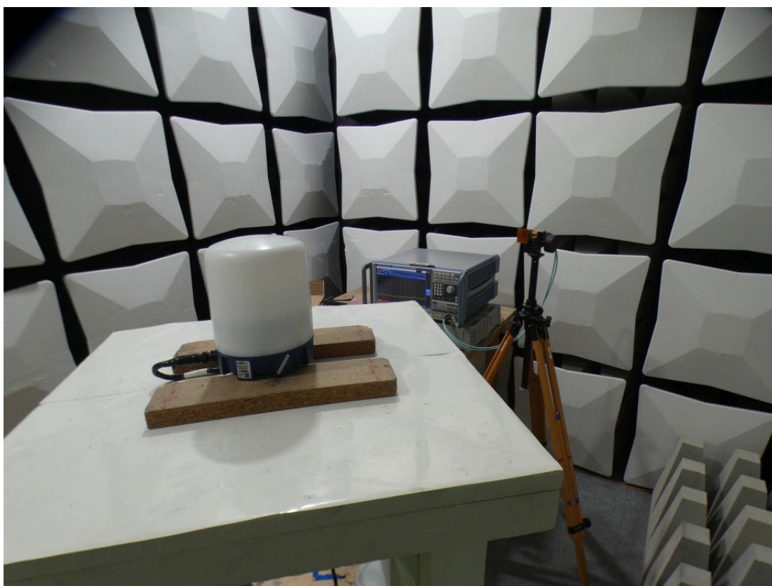
Photo 6: Test setup for radiated measurements (fully-anechoic chamber, > 40 GHz, RSS, Measurement distance: 1m)
