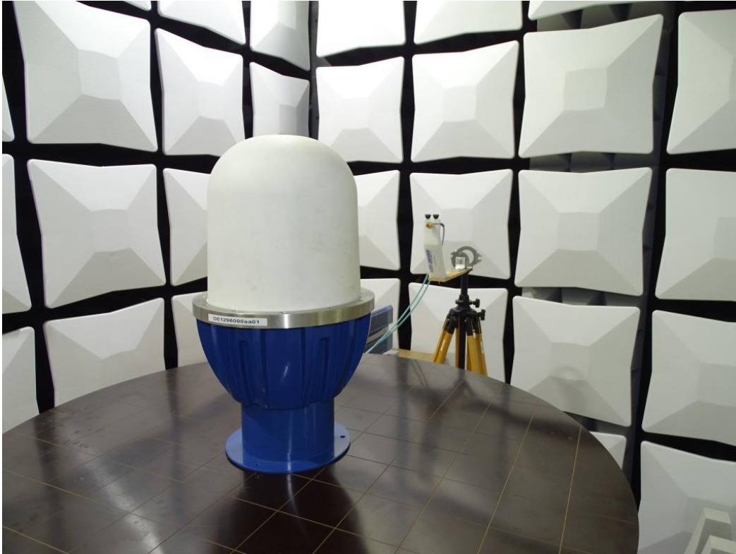
Photo 2: Test setup for radiated measurements
