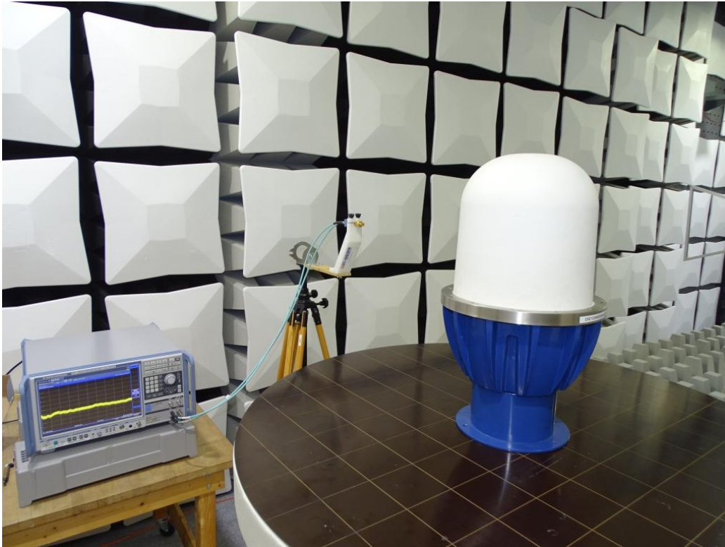
Photo 1: Test setup for radiated measurements
