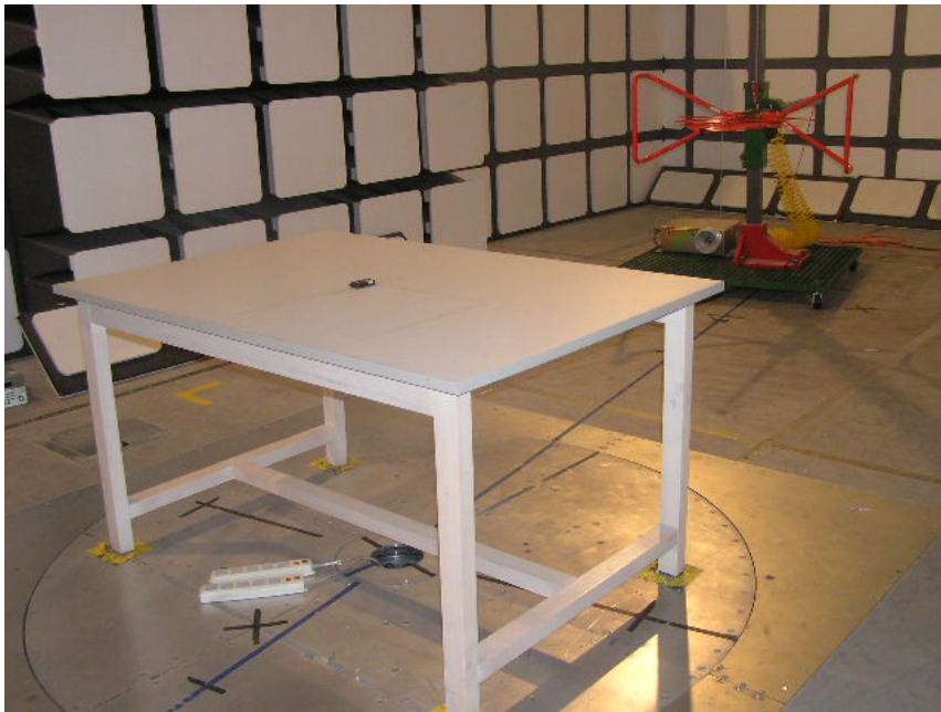
Radiated Emission - Front View
