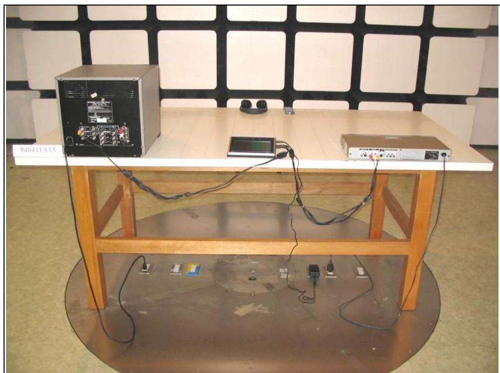
Radiated Emission Test (Car Charger Mode)
