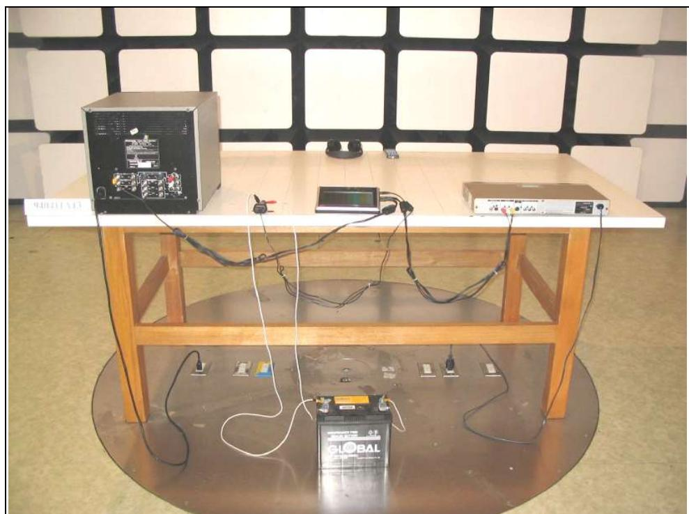
Radiated Emission Test (Battery Mode)
