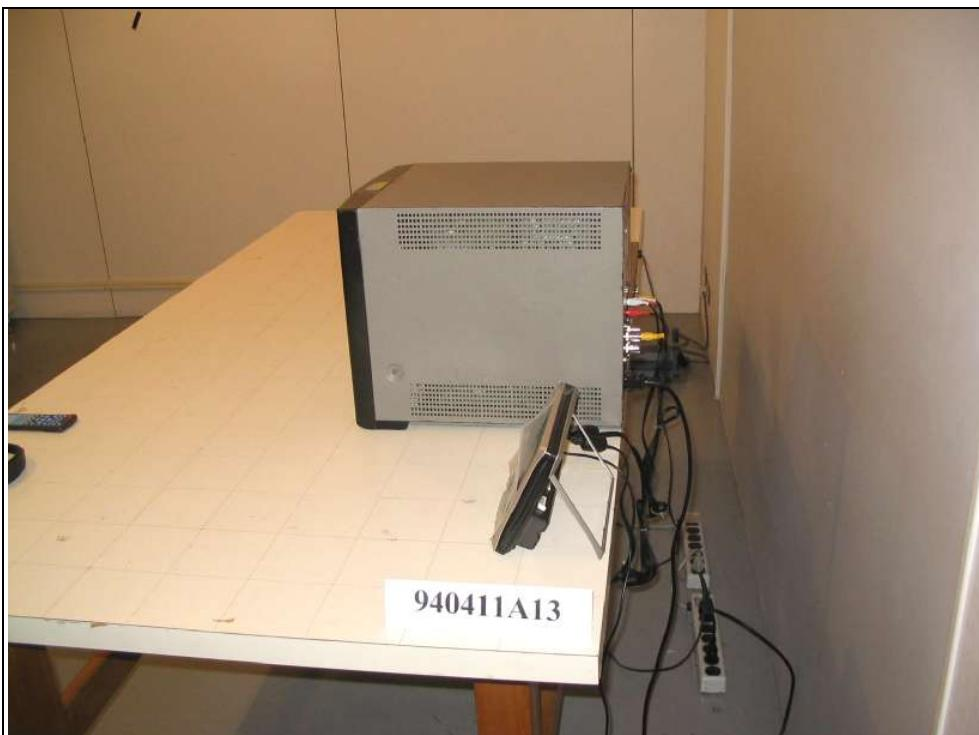
Radiated Emission Test (Adapter Mode)
