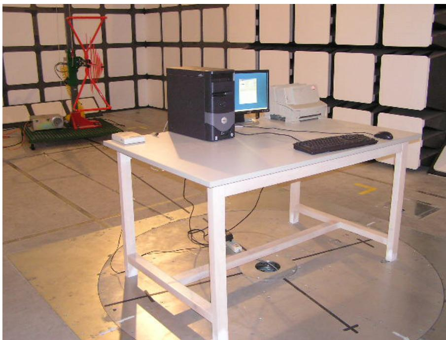
**Radiated Emission - Rear View (30 MHz-1 GHz)**
