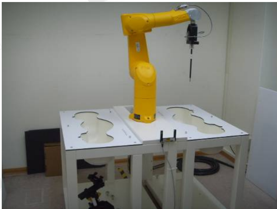
Fig.1 Photograph of the SAR measurement System
