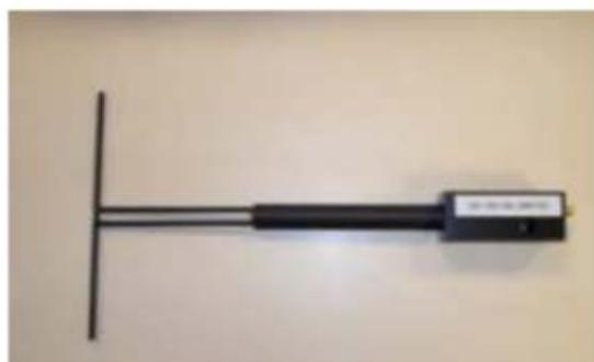
Figure 1 – Satimo COMOSAR Validation Dipole
