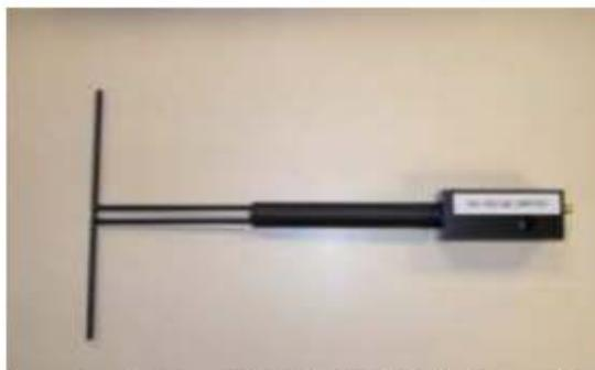
Figure 1 – Satimo COMOSAR Validation Dipole
