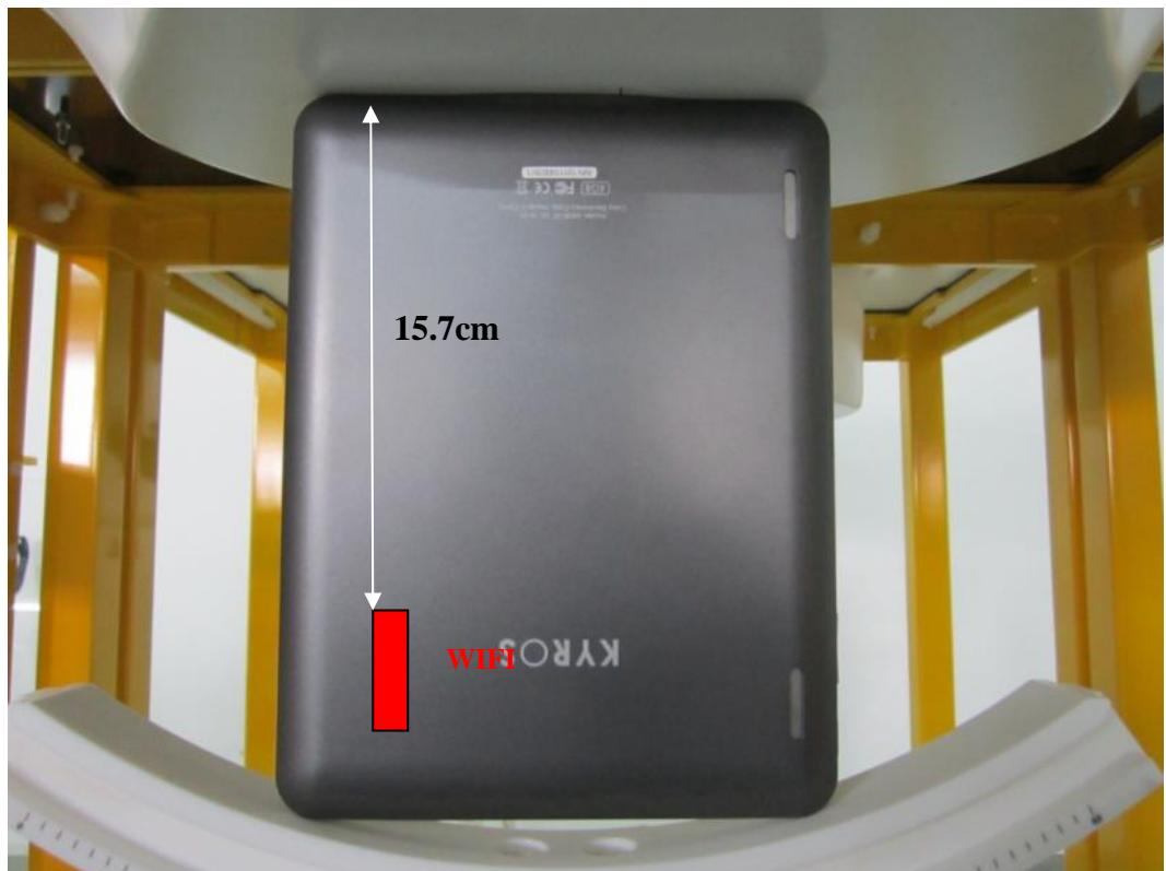
Position E (the distance between WiFi antenna and flat phantom is about 12.5cm. This is not most conservative antenna-to-user distance at edge mode. NO SAR)
