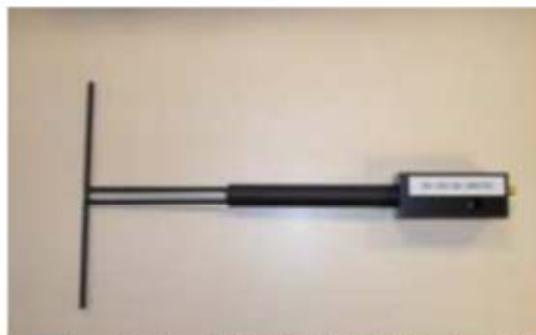
Figure 1 – Satimo COMOSAR Validation Dipole
