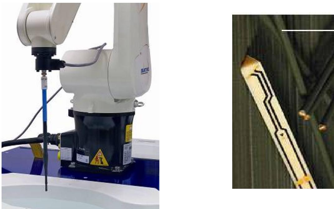
Construction Symmetrical design with triangular Core. Built-in shielding against static charges Calibration in air from 100 MHz to 2.5 GHz. In brain and muscle simulating tissue at frequencies from 800 to 6000 MHz (accuracy of 8%) .
