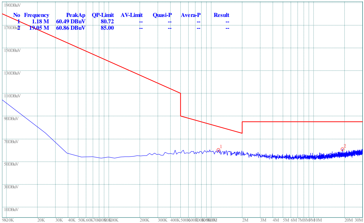
(Plot A.0: 9kHz to 30MHz @ GFSK, channel 0)
