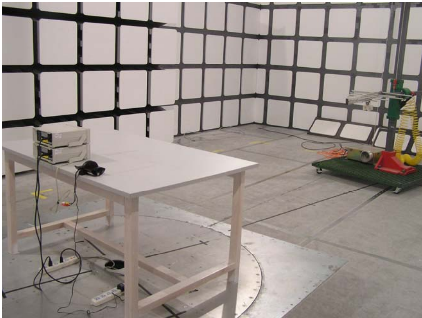
Radiated Emissions-Rear View (below 1GHz)
