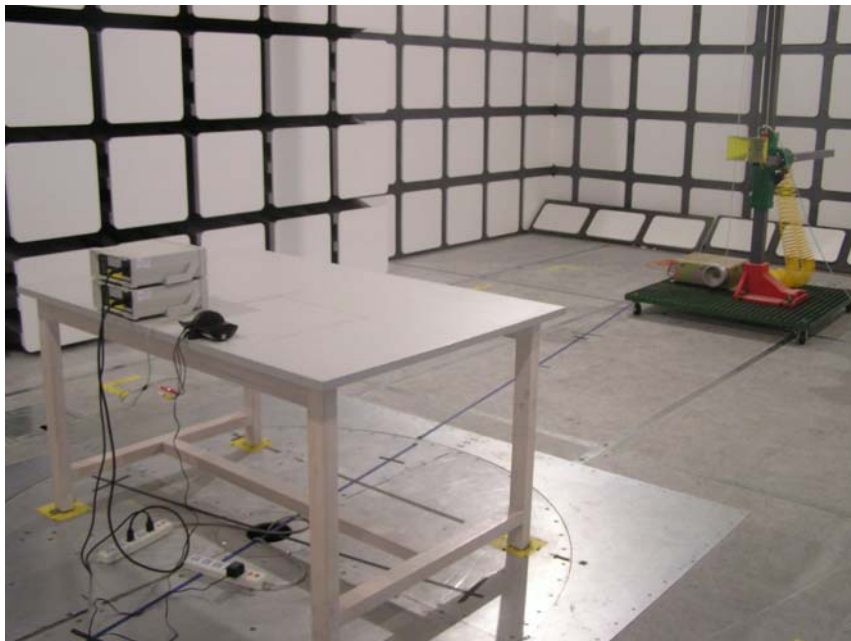
Radiated Emissions-Rear View (above 1GHz)
