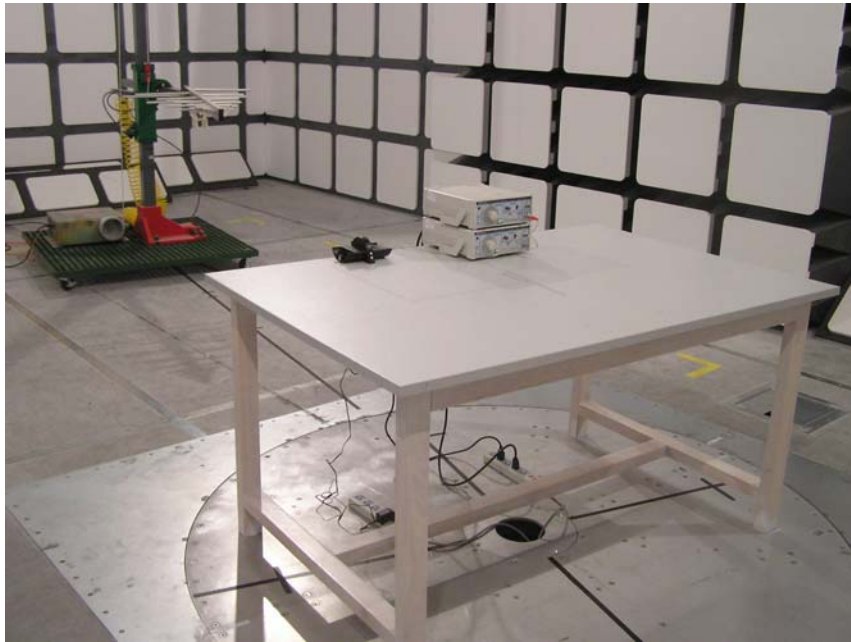
Radiated Emissions-Front View (below 1GHz)
