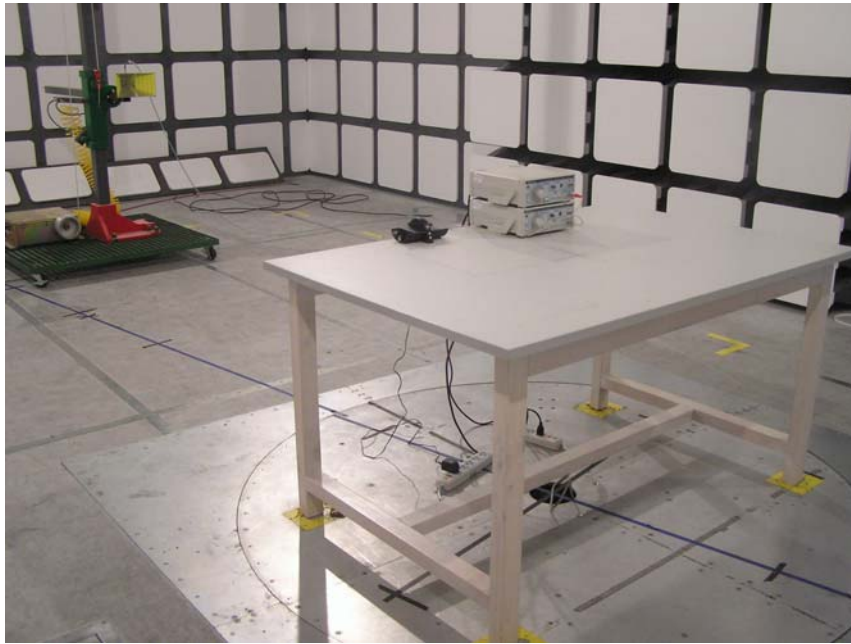
Radiated Emissions-Front View (above 1GHz)
