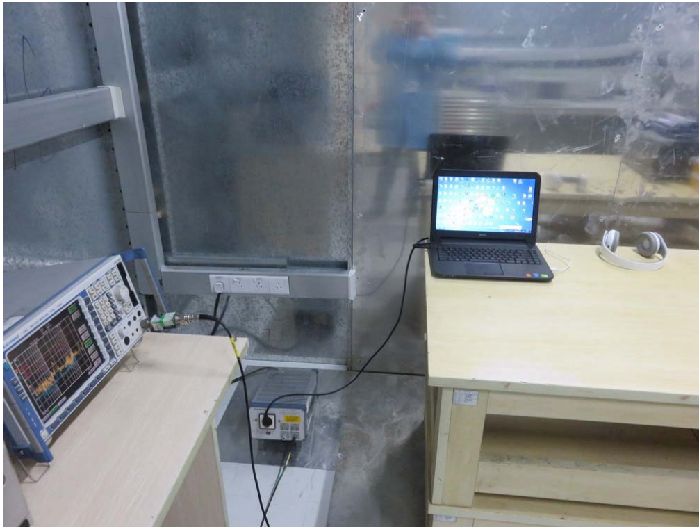
FCC RADIATED EMISSION TEST SETUP
