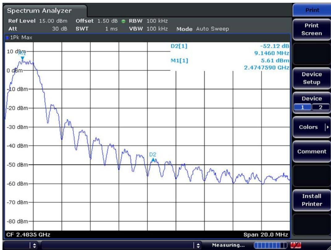
**Band-edges in the restricted band 2310-2390 MHz measurement**
