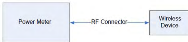
Figure 8.2 Power Measurement Setup
