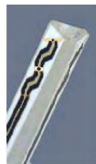
Figure 3.3 Probe Thick-Film Technique
