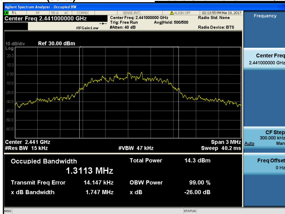
**Occupied Bandwidth (99 %)****Highest Channel &  $\pi/4$  DQPSK**
