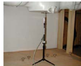
Figure 9.1 Dipole Verification Test Setup Diagram & Photo
