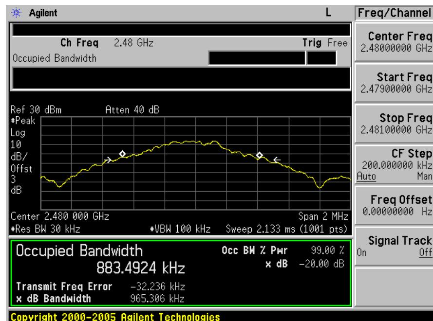
8DPSK \_ Low frequency | 20 dB Bandwidth &amp; Occupied Bandwidth
