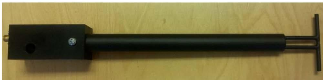
Figure 1 – MVG COMOSAR Validation Dipole
