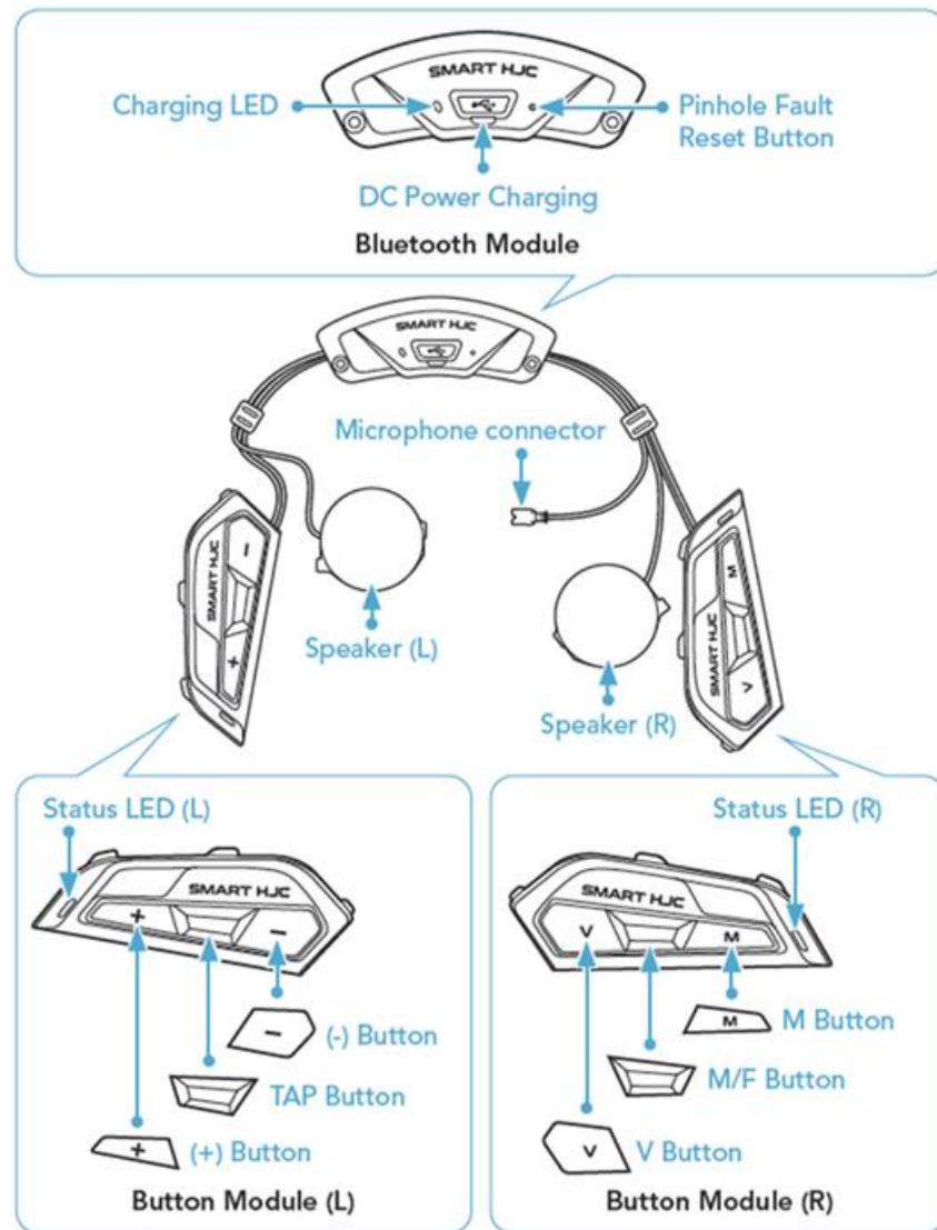
\* Status LED (L) and Status LED (R) operate simultaneously.
